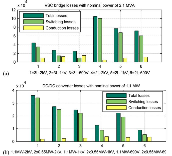
Figure 4. Power losses with nominal power for the (a) VSC bridges, (b) DC/DC converter power stages.
