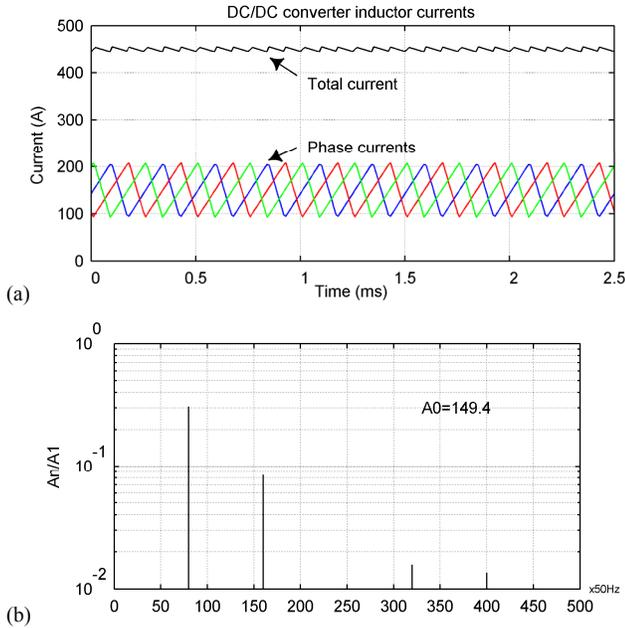
Figure 5. Currents of the single 1.1 MW DC/DC converter inductors with nominal power. (a) Inductor phase currents and total current, (b) normalized amplitude spectrum of inductor phase-A current.
