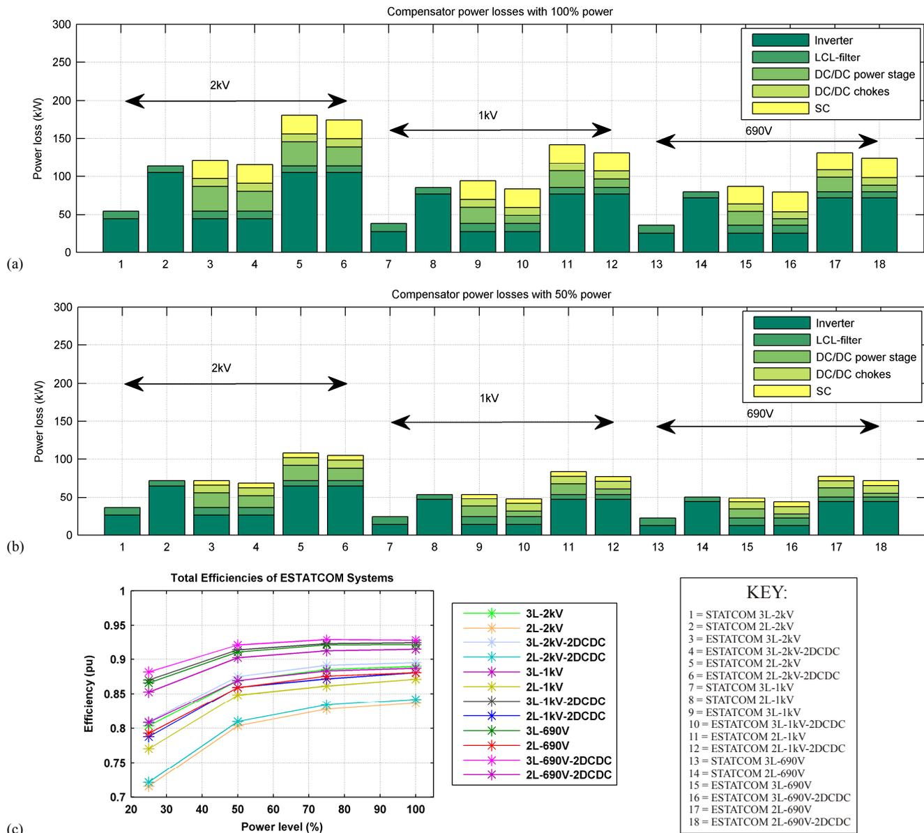
Figure 7. System losses with (a) 100% power, (b) 50% power, and (c) ESTATCOM total efficiencies with power levels of 25 % to 100 %.
