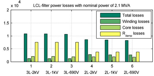
Figure 3. LCL-filter power losses with nominal power.
