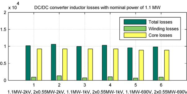
Figure 6. DC/DC converter inductor losses with nominal power of 1.1 MW.
