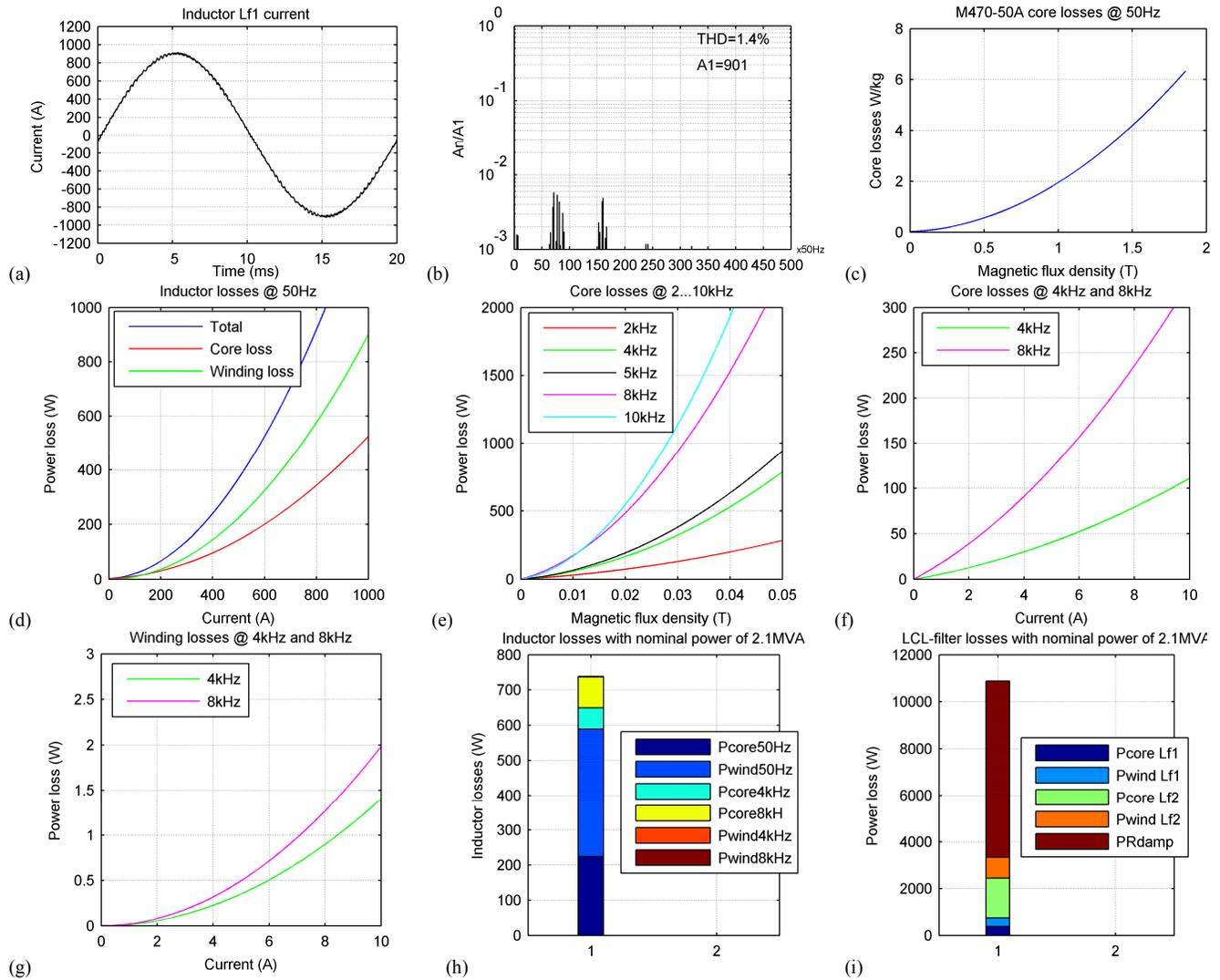
Figure 2. Power loss modelling of inductor  $L_{f1}$  in the 3-level 2 kV system. (a) Inductor current, (b) normalized amplitude spectrum of inductor current, (c) characteristic core loss curve for M470-50A electrical steel, (d) inductor core- and winding losses at 50 Hz, (e) high frequency core loss curves for M470-50A electrical steel, (f) high frequency core losses, (g) high frequency winding losses, (h) inductor total losses, (i) LCL-filter total losses.
