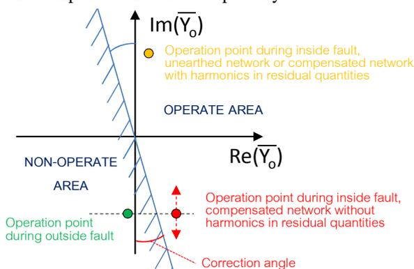
*Fig. 1* Operation characteristics of multi-frequency neutral admittance protection, which is valid both in compensated and unearthened networks.
