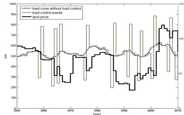
Figure 3. Example of spot price-based load control for 248 customers with direct electric heating loads during 60 hours
