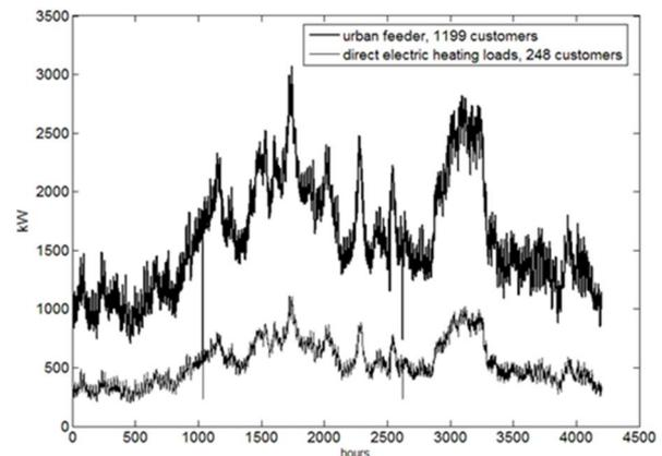
Figure 4. Load curve without load control actions
