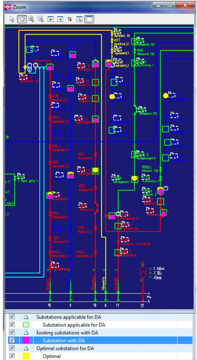
**Figure 2.** The illustration of applicable secondary substations for DA, existing DA substations and suggested optimal distribution automation secondary substations on network diagram.
