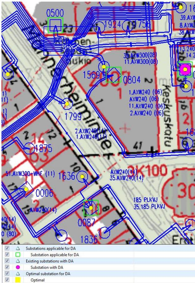
**Figure 3.** The illustration of applicable secondary substations for DA, existing DA substations and suggested optimal distribution automation secondary substations on network map.
