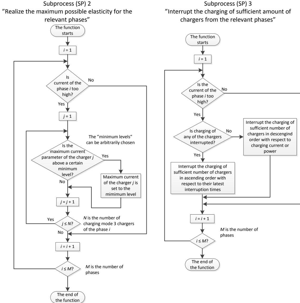
Fig. 4. Functions “Realize the maximum possible elasticity for the relevant phases” and “Interrupt the charging of a sufficient number of chargers from the relevant phases”.
