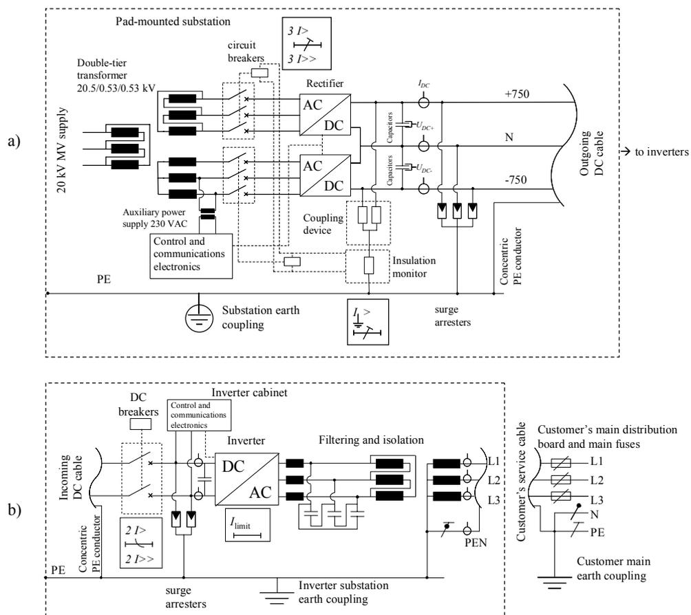
Fig. 3. Main power circuits and protection devices at a) the rectifier and b) the CEI side of the system. There are three similar CEIs in the setup.
