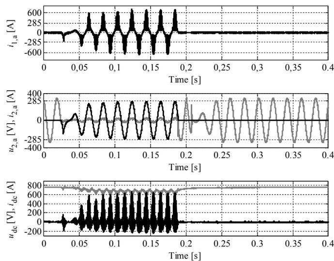
Fig. 4. Measured short-circuit response using a 285 Apeak (200 Arms) current reference.
