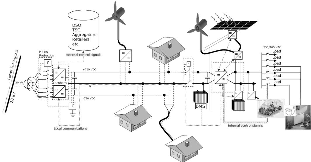
Fig. 1. Example of an active LVDC electricity distribution system with DG and energy storages.
