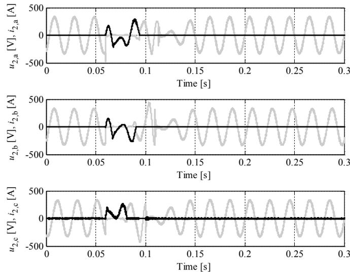
*Fig. 5. Short-circuit currents (black) and phase voltages (grey) during single-phase fault in phases L1 (top), L2 (middle), and L3 (bottom). Protection device used was C20 circuit breaker.*
