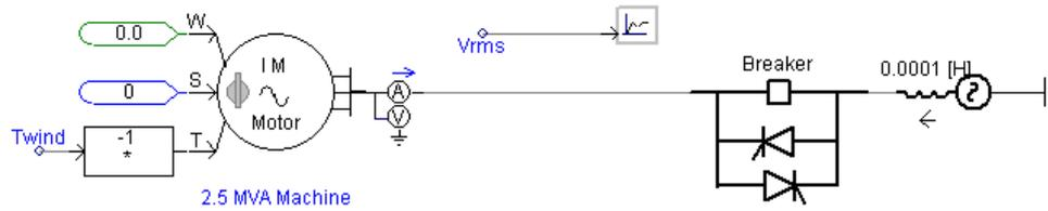
Figure 2. Induction machine with wind turbine model input. [19]
