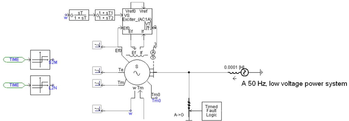
Figure 4. Synchronous machine with wind turbine model input. [19]
