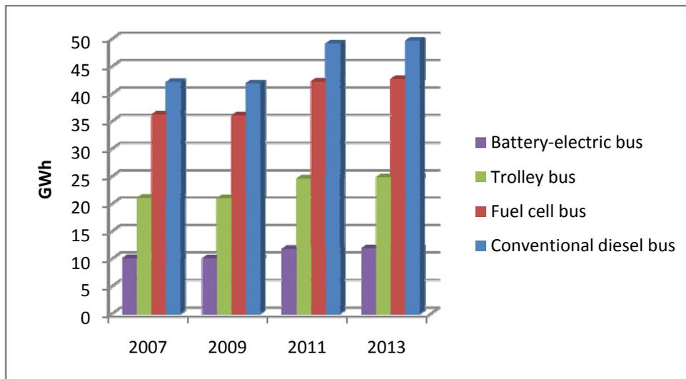
Figure 4: Energy consumption estimates for various vehicle types in internal bus transportation in Vantaa
