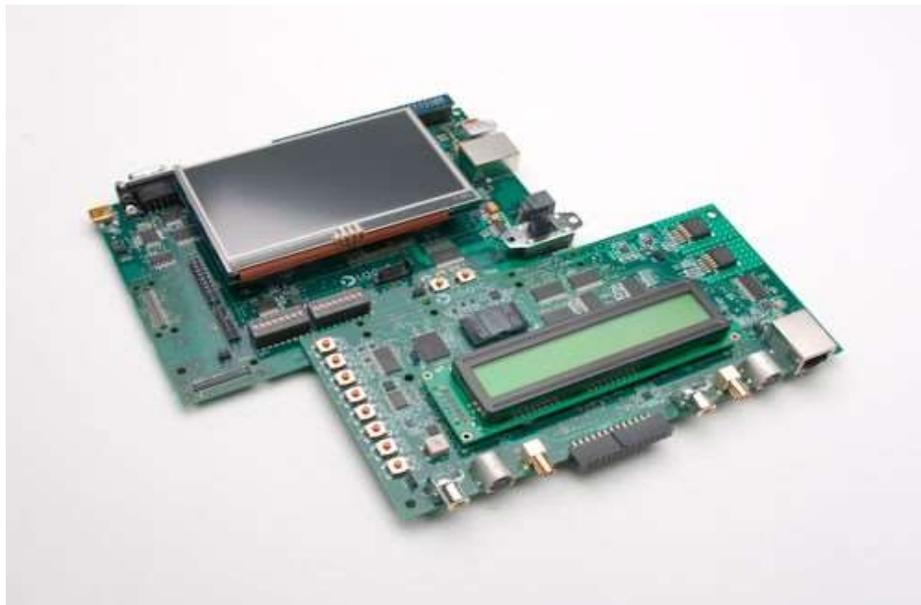
Fig. 1: OMAP-L138 EVM interfaced with UI board
