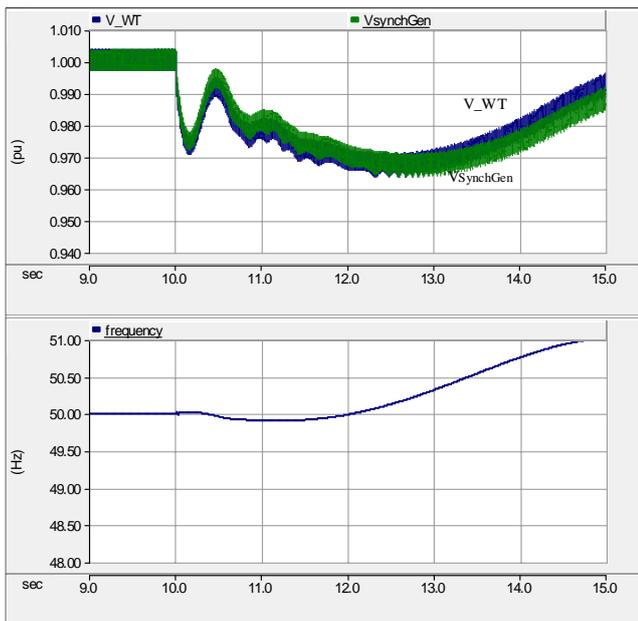
Fig. 9. Voltages and frequency from the PCCs when a deficit of 64kW and 60kVar was present before the islanding. The RPV method was disabled.
