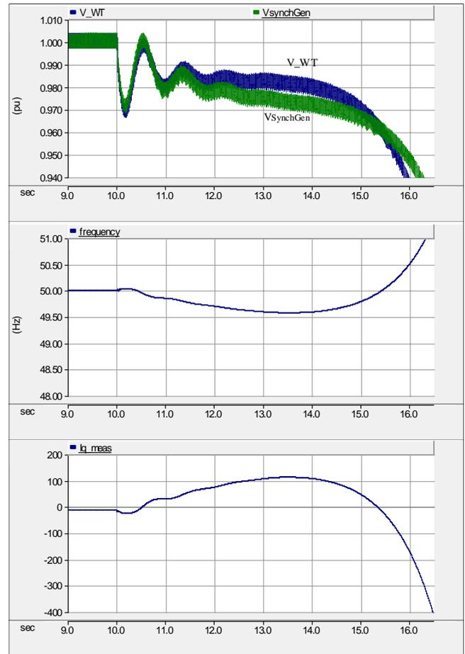
Fig. 10. Voltages and frequency from the PCCs when a deficit of 64kW and 60kVar was present before the islanding. The Iq gain was set to 300A/Hz.
