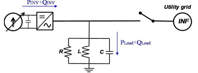
Fig. 2. A simple circuit for islanding detection analysis.
