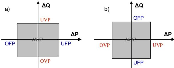
Fig. 1. Non-detection zone for voltage and frequency based LOM protection when the DG unit in question is a) directly connected b) converter coupled.
