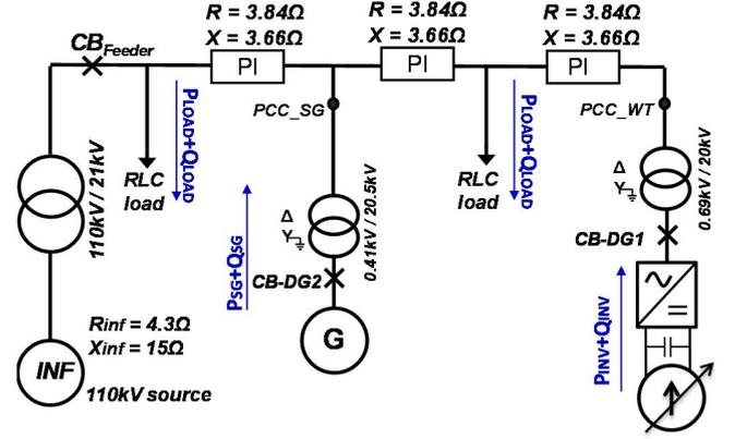
Fig. 3. The general structure of the utilized simulation model.
