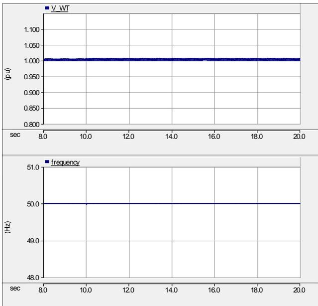
Fig. 4. Voltage magnitude and frequency when only the FCWT was connected and the  $I_q$  gain of the RPV method was set to 0.01A/Hz.
