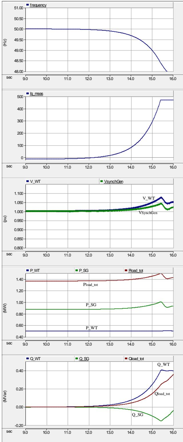
Fig. 7. Voltage frequency, q-component of inverter current and voltage magnitude when both DG units were connected in parallel and the frequency droop  $I_q$  gain value was set to 300A/Hz.
