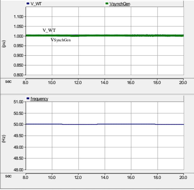
Fig. 6. Voltage magnitude of the PCCs of the DG units and voltage frequency
