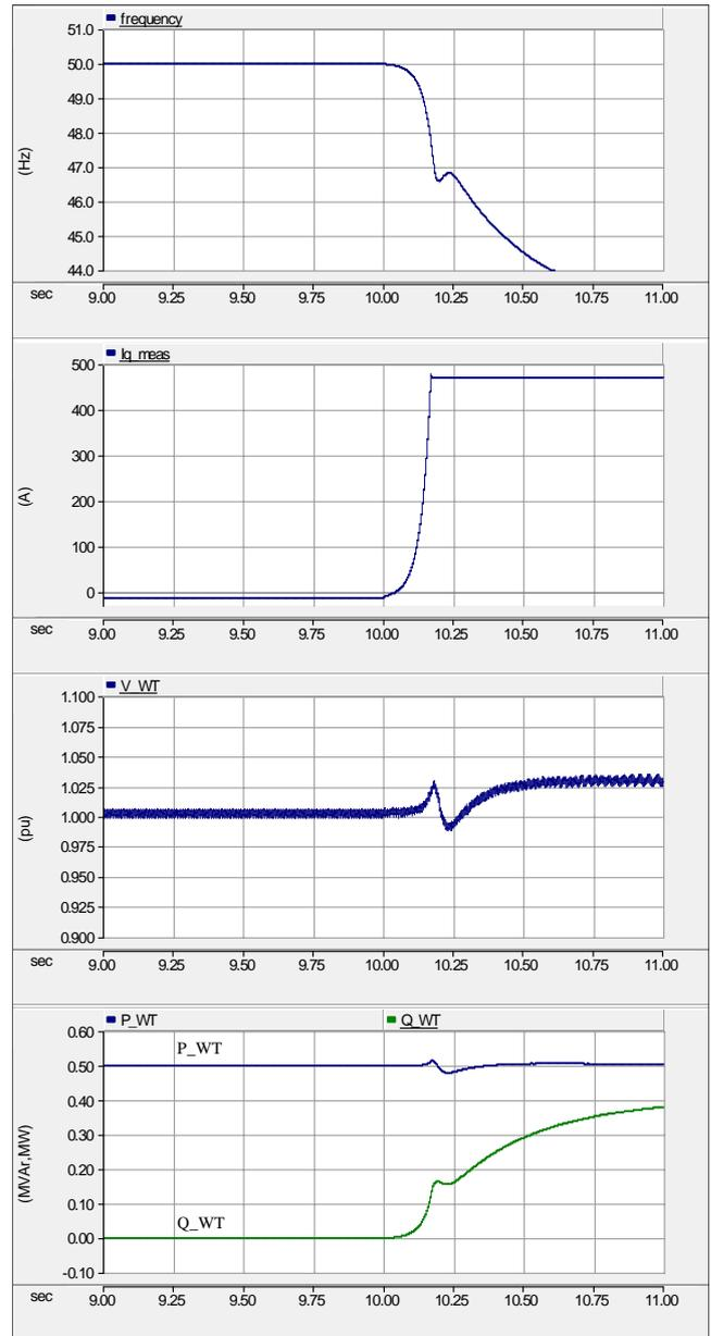
Fig. 5. Voltage frequency, q-component of inverter current and voltage magnitude when only the FCWT was connected and the  $I_q$  gain value of the RPV method was set to 300A/Hz.
