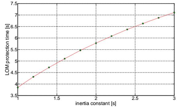
Fig. 8. The effect of inertia constant of synchronous generator on LOM detection.
