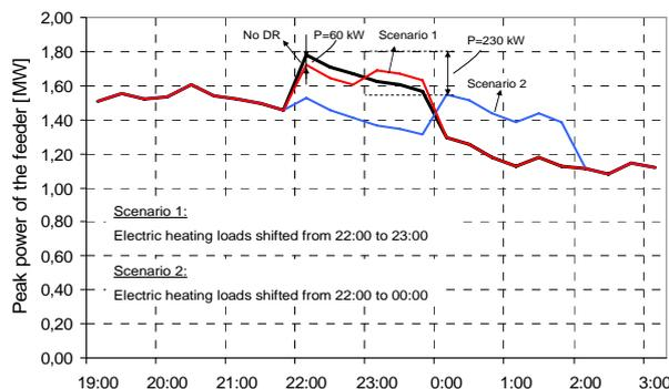
Fig. 3. Impact of load control on the load curve shape. 60 kW are shifted for 1 hour and 256 kW are shifted for 2 hours.
