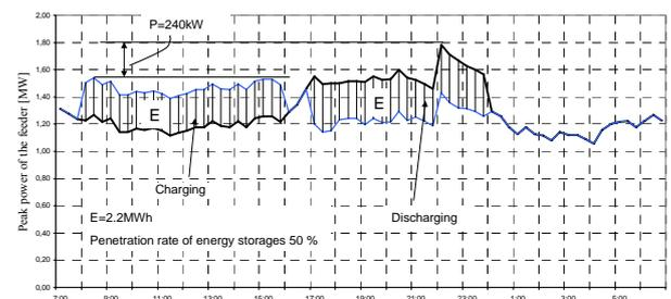
Fig. 4. Impact of energy storages on the load curve shape.
