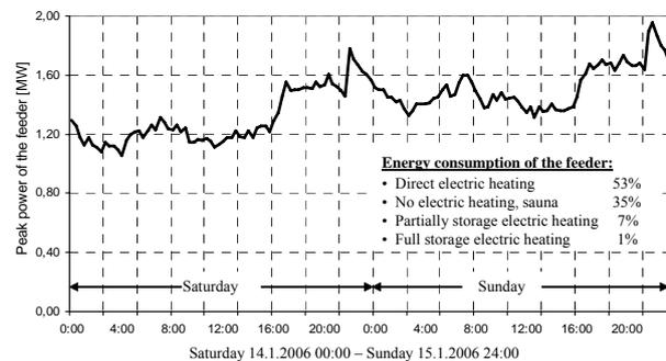
Fig. 2. Load curve of the case feeder.
