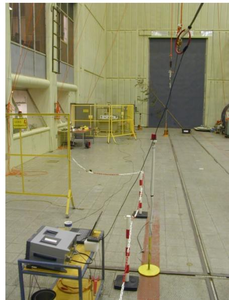
Figure 1. On-line Single-phase PD measuring set-up using Rogowski coil
