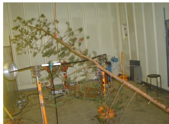
Figure 2. On-line Single-phase PD measuring set-up using Pearson coil
