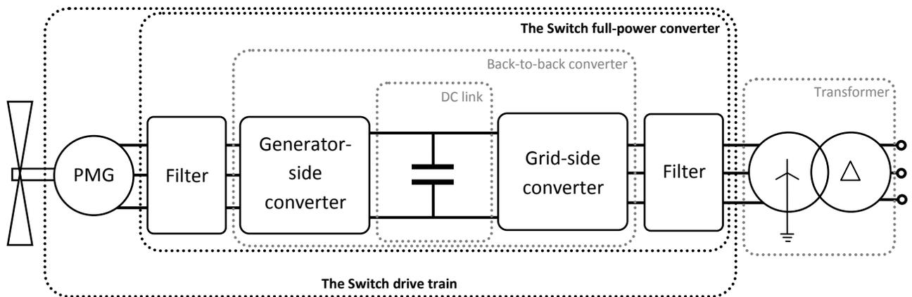
Figure 1: A block diagram of the full-power converter for a wind turbine based on a permanent magnet generator (PMG). The generator transforms the wind energy into electrical energy. The energy flow is controlled by a back-to-back converter that contains two IGB-transistor bridges. The filters clean the electrical signal from noises harmful for the PMG and a grid load, connected to the system through a transformer.
