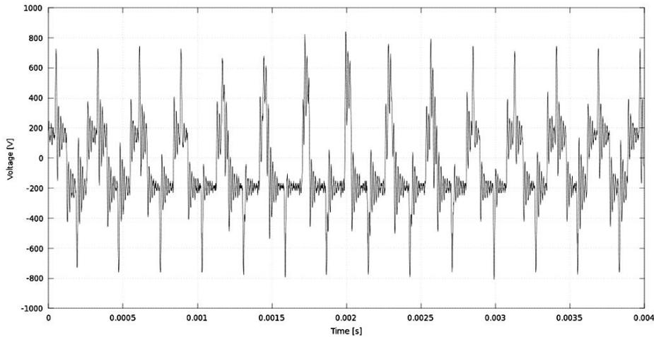
Figure 3: Common-mode voltage generated by the grid-side converter, which affects the generator phase-to-ground voltage. This voltage is highly oscillatory because of the  $LC$  resonances between phase inductances and stray capacitances present in a generator and, if not taken into account during system design, can cause unexpected generator failures.
