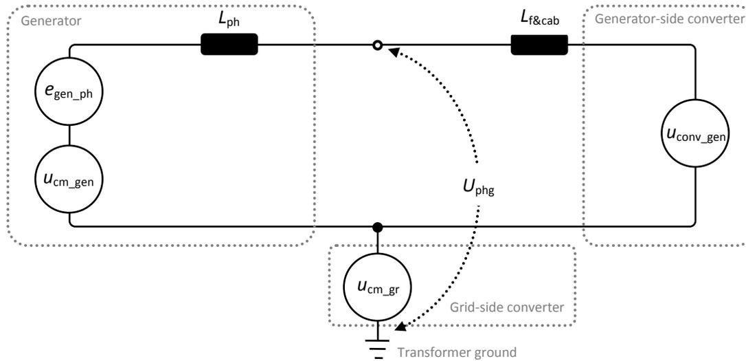
Figure 2: A simplified electrical circuit of the back-to-back converter system, which describes the phase-to-ground voltage generation in a full-power converter. The phase-to-ground voltage is thus a combination of the back-to-back converter voltages, which depend on the relation between the generator inductance  $L_{ph}$  and the sum of the generator-side filter and cable inductances  $L_{f\&cab}$ .
