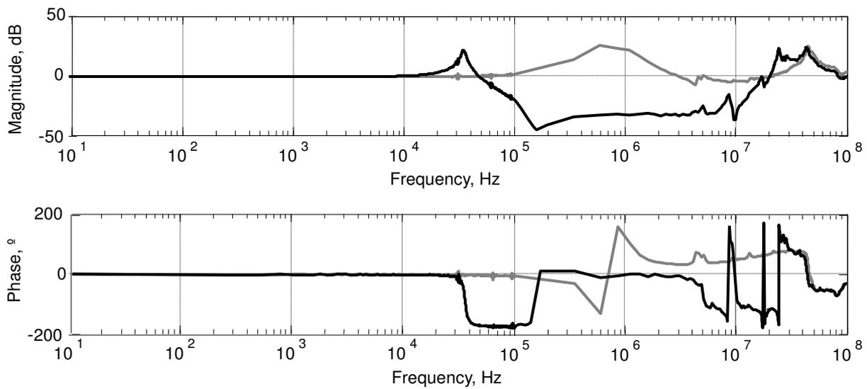
**Fig. 3.** Frequency responses of HLCF: — – Terminal 1 earthed, - - - Terminal 2 earthed.
