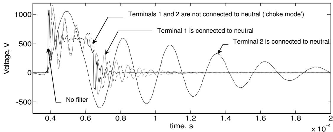
**Fig. 4.** Time domain measurements of the hybrid *LC* filter.
