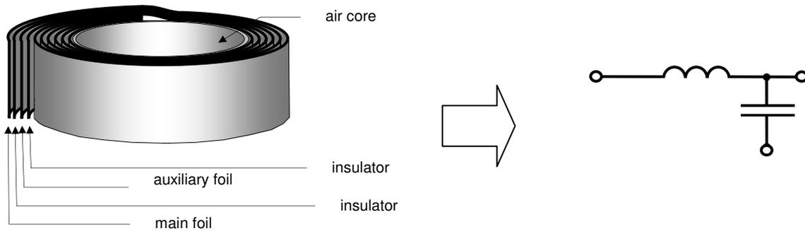
**Fig. 1.** Single-phase column of the proposed hybrid  $LC$  filter.
