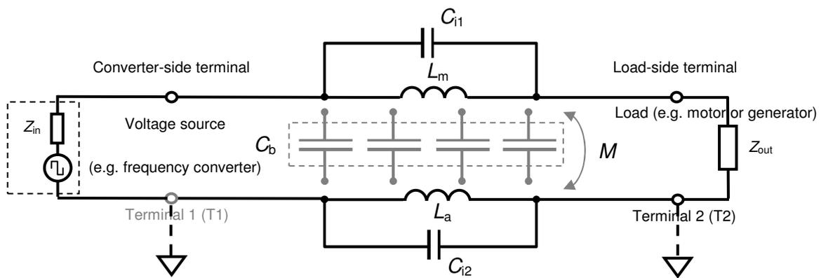
**Fig. 2.** Lumped presentation of the hybrid  $LC$  filter.
