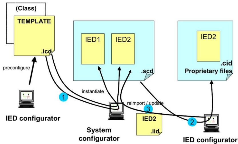
Figure 3. Modification process [IEC09].
