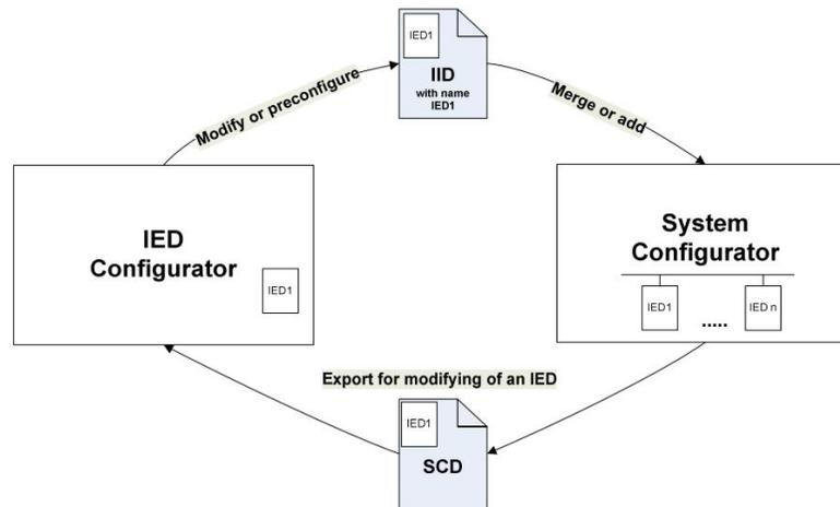
*Figure 1. Two main levels – IED Configurator and System Configurator. Updates possible via IID files [IEC09].*
