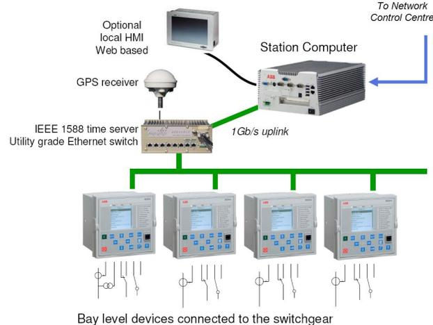
*Figure 5. Overall setup of centralized protection and control system*
