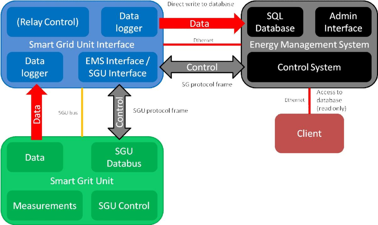
Fig. 2. Concept of the communication structure between the EMS and the SG-units.
