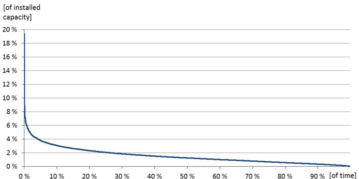
Figure 6 Duration curve of wind power intra-hour changes from hourly average value as % of capacity in West Denmark in 2012 (Data source: Energinet.dk 2013).
