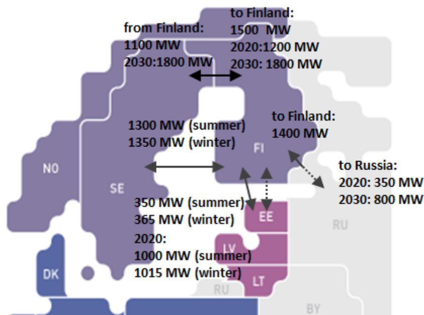
Figure 1 Cross-border transmission capacity in Finland today and assumptions for 2020 and 2030 (Modified from the data sources: ENTSO-E 2012a and ENTSO-E 2012b, p. 49).
