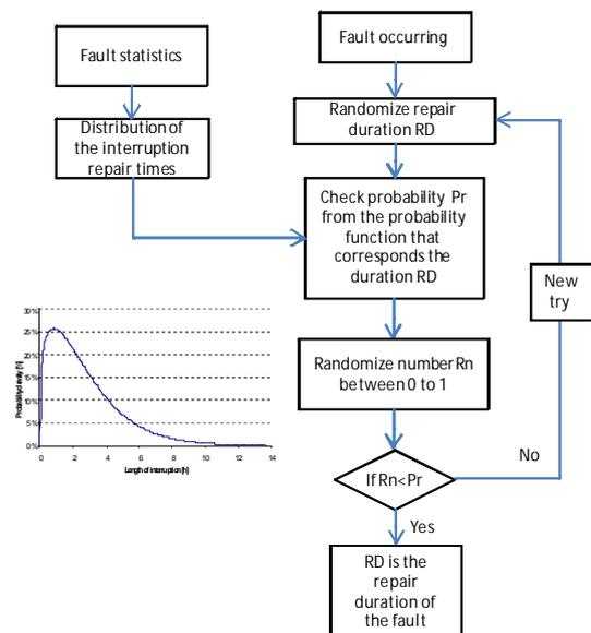
**Figure 9:** Fault repair time algorithm for each fault occurrence.
