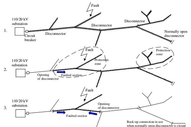
**Figure 4:** Fault isolation process. In the first step, the circuit breaker is operated. In the second step, the disconnector in front of the fault is opened. In the third step, the disconnector after the fault is opened and the back-up switch is closed [11].
