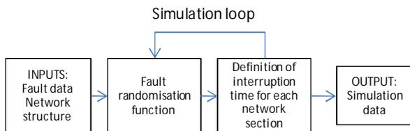
**Figure 1:** The principle of the simulation sequence.
