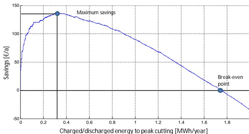
Fig. 7. Savings vs. needed battery capacity (charging/discharging).
