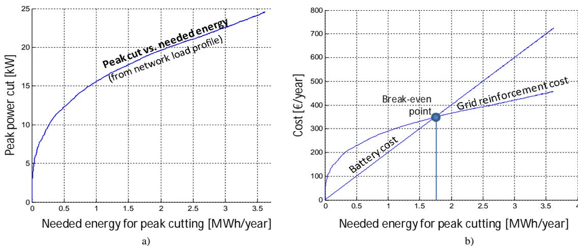
Fig. 6. a) Peak cut vs. needed energy (taken from the network load profile). b) Economic limit for peak cut.
