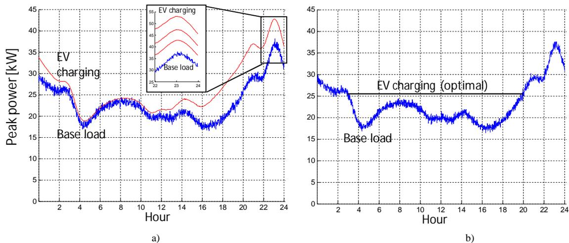
Fig. 3. Load curve when (a) no intelligence and (b) intelligence is implemented into charging.
