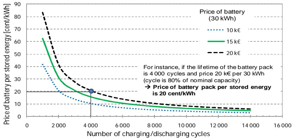
Fig. 5. Price of batteries (30 kWh) compared with their lifetime (number of charging and recharging cycles).
