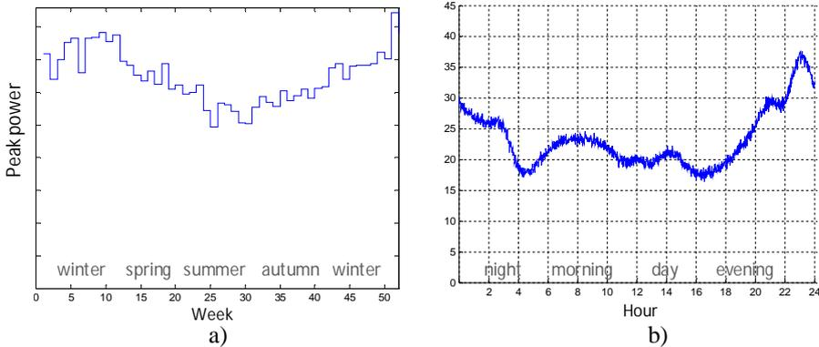
Fig. 2. Annual (a) and daily (b) load curves of residential customers (electric heating with a water storage).
