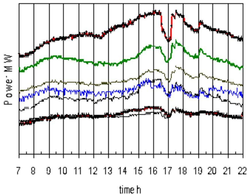
Figure 1. Measurements from the controlled substations in direct load control field test on 24 December 1996, when outdoor temperature was  $-26^{\circ}\text{C}$ .
