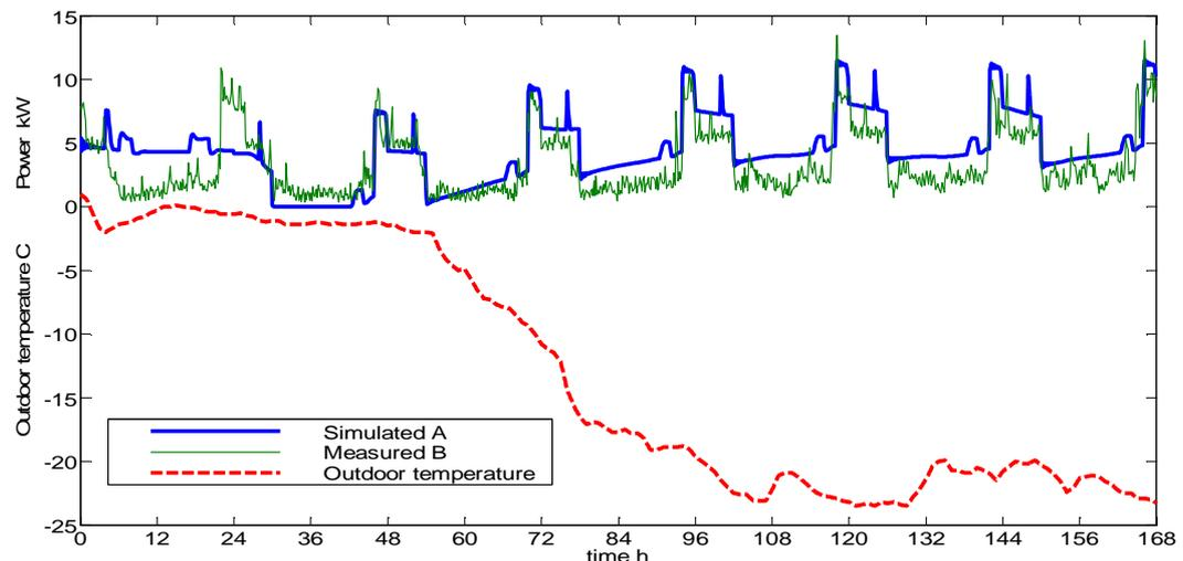
Figure 13. Measured and simulated loads of a row house apartment in Time-of-Use control in Helsinki area. [Koponen 2006]
