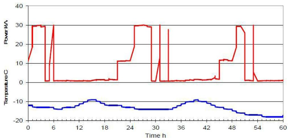
Figure 2. Measurements of a full storage heating house in Time of Use control in 1997. [a sample of measurement data provided by Hannu Pihala]
