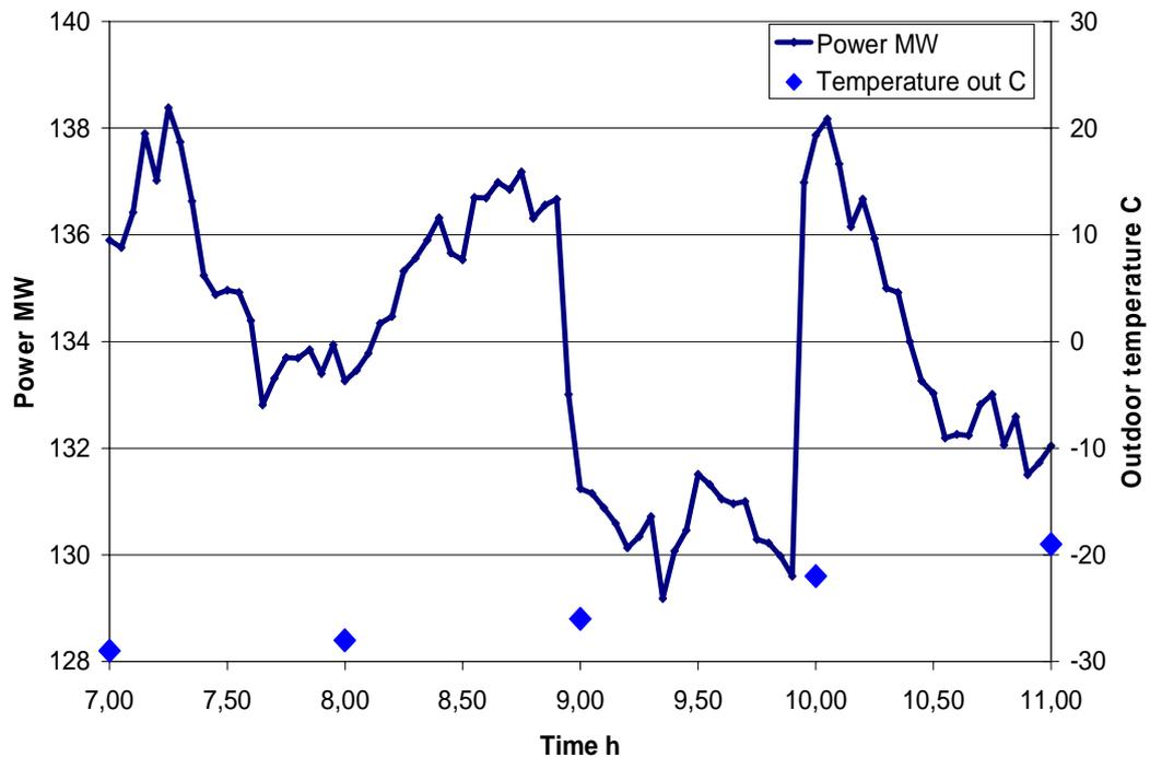
Figure 8. Response measured at direct load control field test at E.ON Kainuu.
