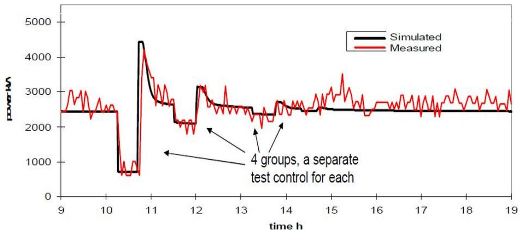
Figure 11. Load control responses measured from substations at two skiing resorts and the responses of the simple physically based model [Koponen 1997].
