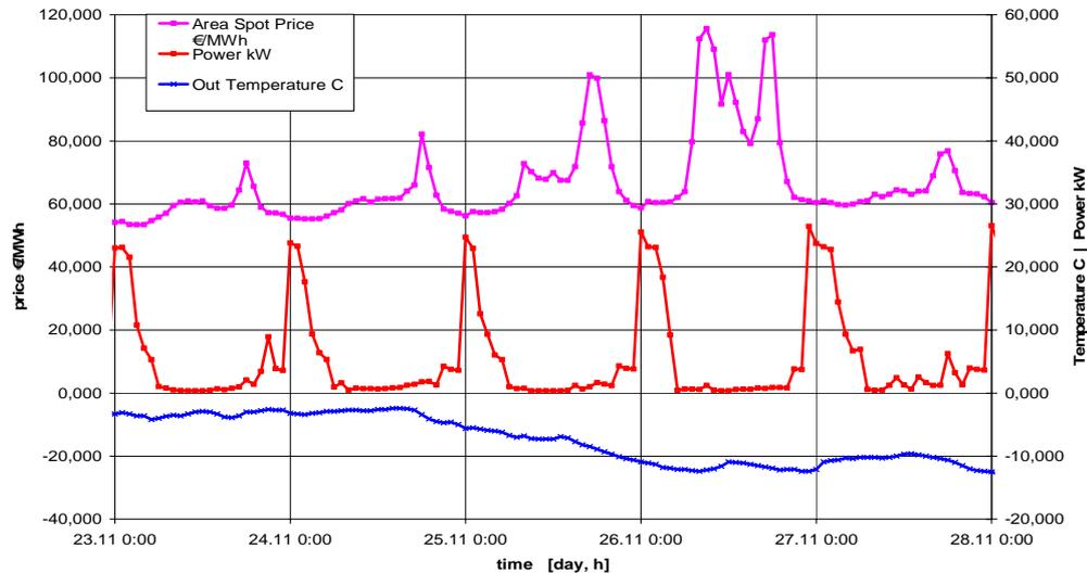
Figure 3. Measurements of a full storage heating house in November 2010.
