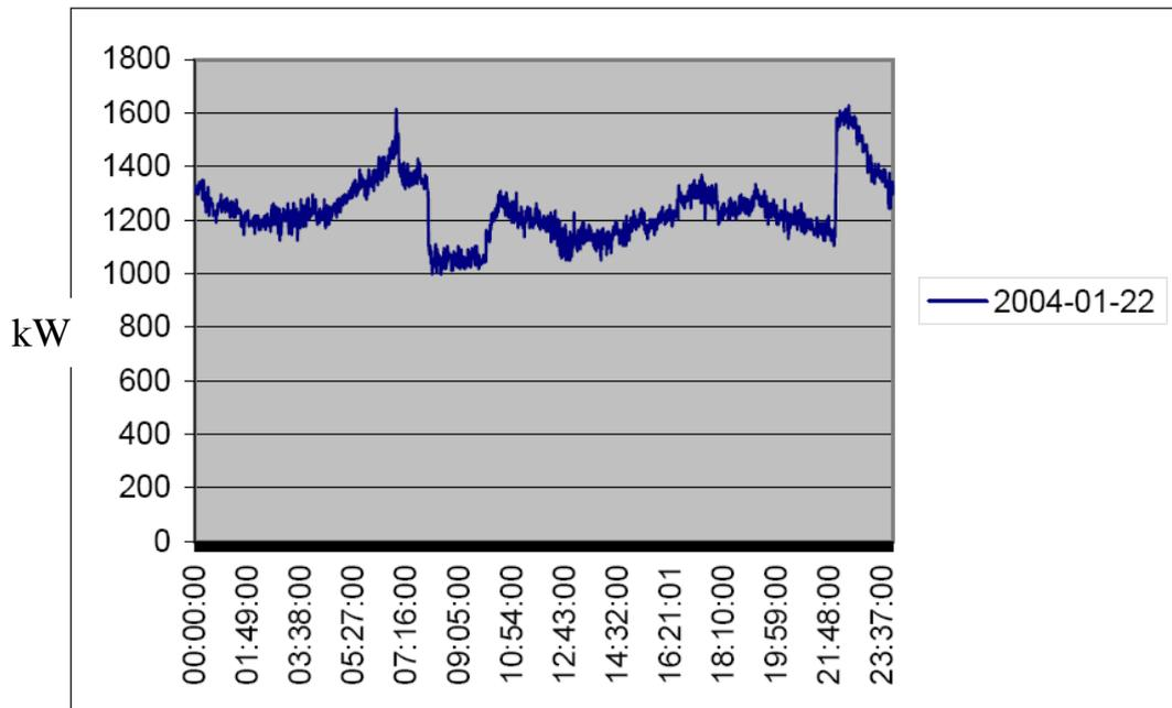
Figure 5. Direct load control experiment in Sweden 22 January 2004. Load reduction is about 280 kW. [ Lindskoug 2006 ]
