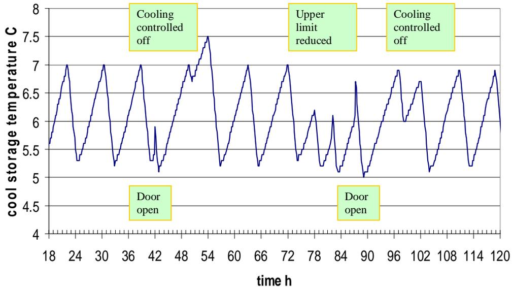
Figure 9. A measurement of cool storage temperature and its response to two load control actions.
