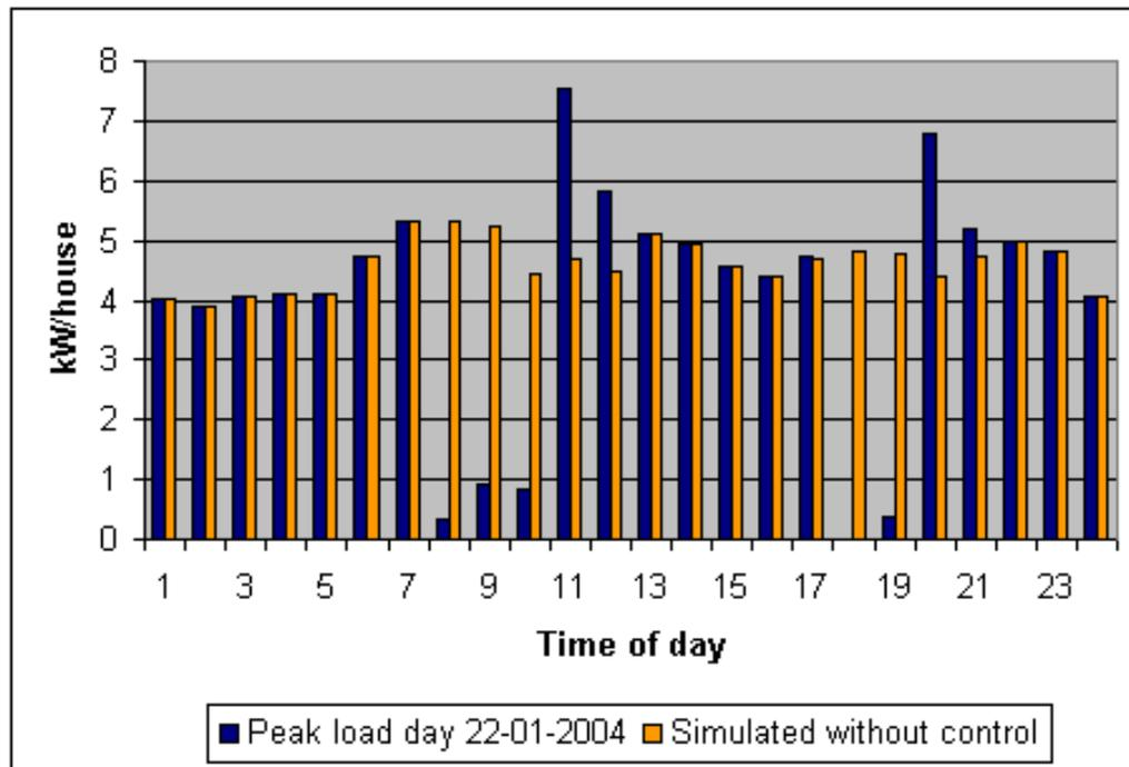
Figure 4. Control responses of a Danish electrically heated house during the peak load day 22 January 2004.
