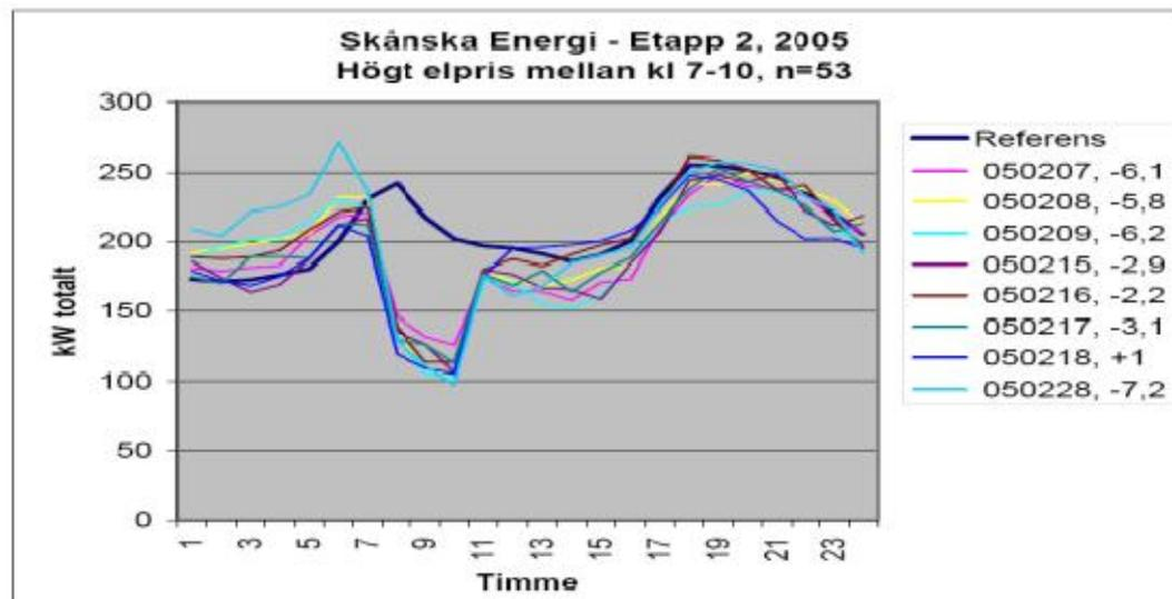
Figure 6. Price control experiment in Sweden in February 2005. Load reduction is about 280 kW. . [ Lindsoug 2006 ]
