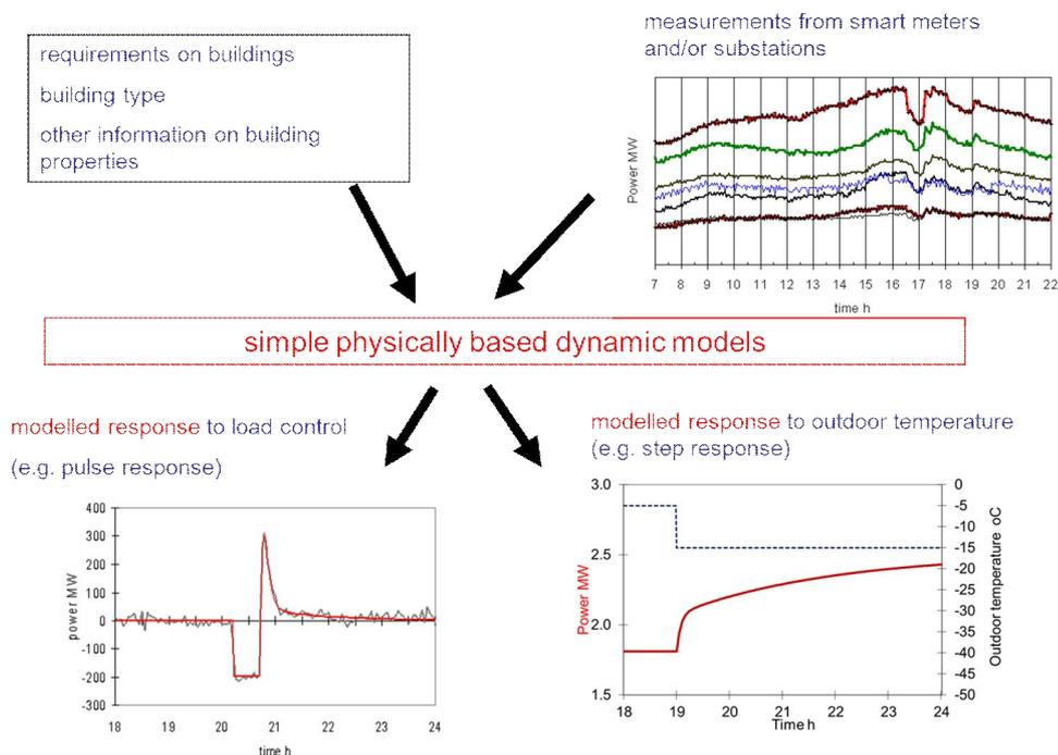
Figure 10. The responses to outdoor temperature and load control are modelled using simple physically based models based on information on building properties and measured data from different sources.
