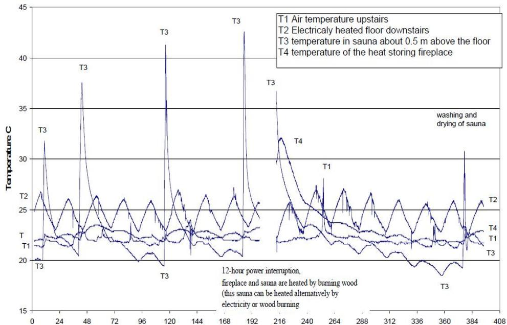
Figure 12. Temperature measurements from a detached house in Helsinki area. [Koponen 2006]
