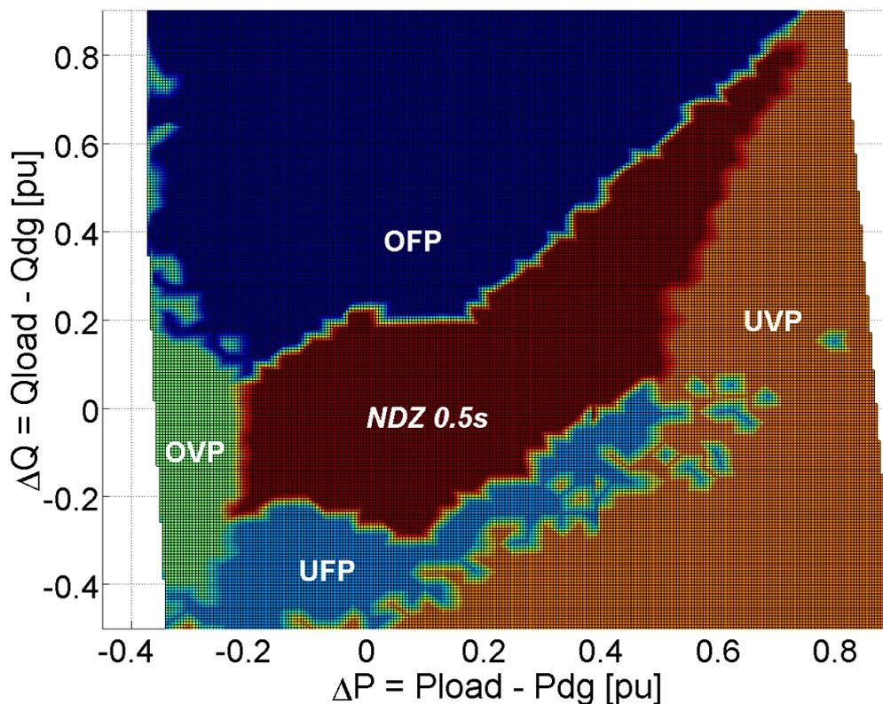
Fig. 7. The NDZ when the protected unit was the FCWT which was operated in voltage droop mode (5% deadband)
