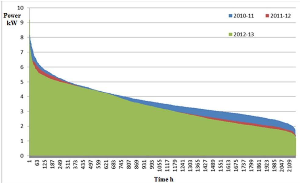
Fig. 7. Temperature corrected load duration curves between December-February in 2010-2013
