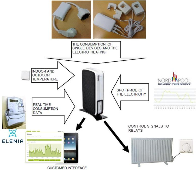
Fig. 2. The basic concept of the pilot HEMS solution [Emmi #]
