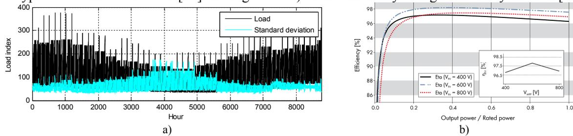
**Figure 4.1 Load behaviour of a Finnish customer, having no electric heating and an electric heated sauna a) [17] and efficiency of commercial SMA solar inverter b) adapted from: [18].**
