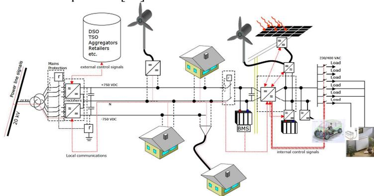
Figure 2.1 Example of the bipolar  $\pm 750$ VDC, earth isolated (IT) LVDC system setup with DERs [10].
