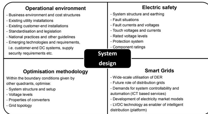
Figure 2.2 LVDC distribution system design aspects
