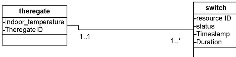
Figure 2.1 ThereGate and Switch class
