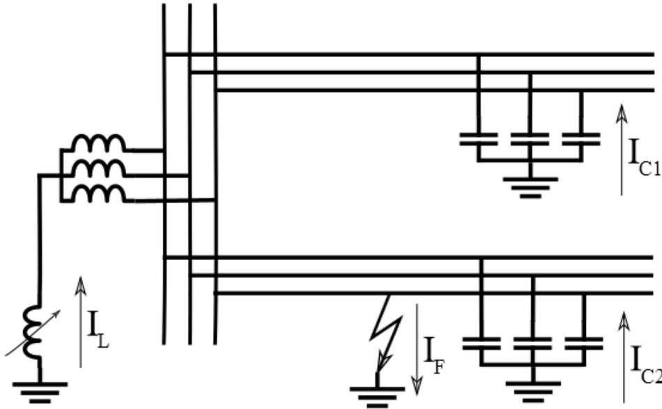
**Figure 3.** Earth fault in resonant earthed network.
