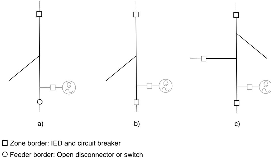
**Figure 2.** Defined basic protection zones: a) radial, b) ring, c) mesh. Also the optional DG is shown. Loads along the feeder are not shown.
