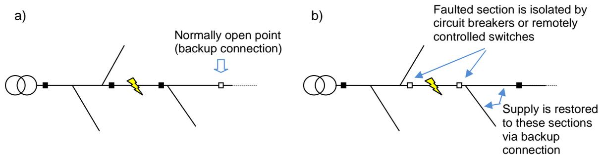
**Figure 1.** Self-healing by using a backup connection. a) Fault occurs. b) Faulted section is isolated and backup connection is closed.
