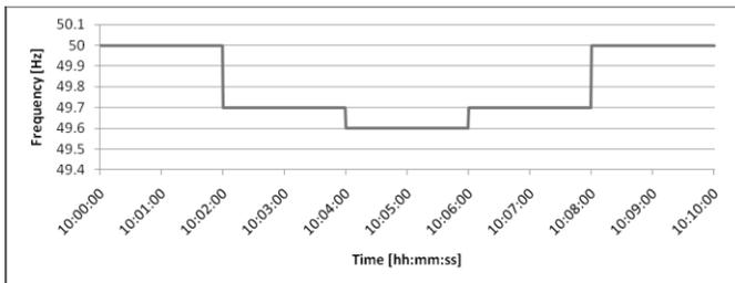
Fig. 3. Predefined frequency disturbance data.
