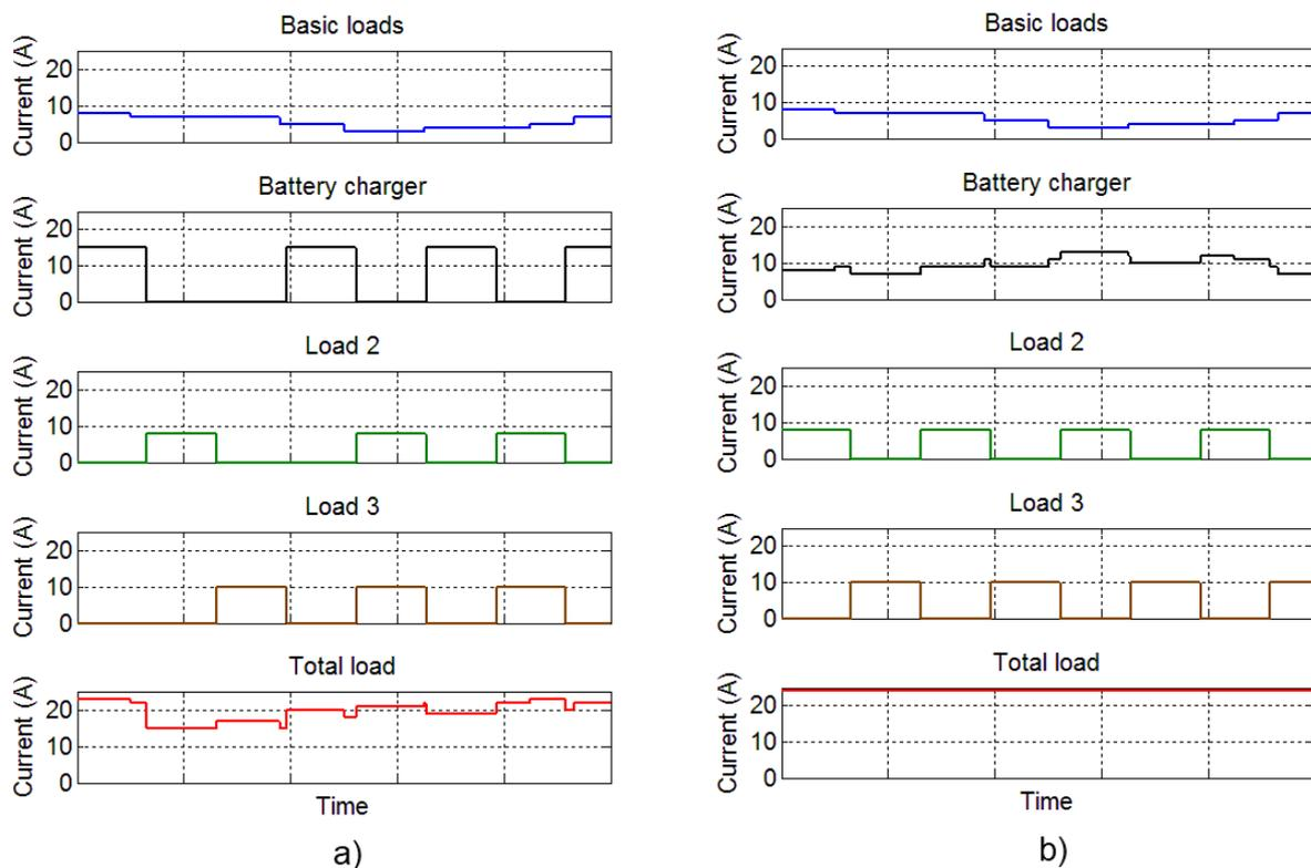
**Fig. 6.** Simplified principles of the two different current restriction methods which use connection point current measurement
