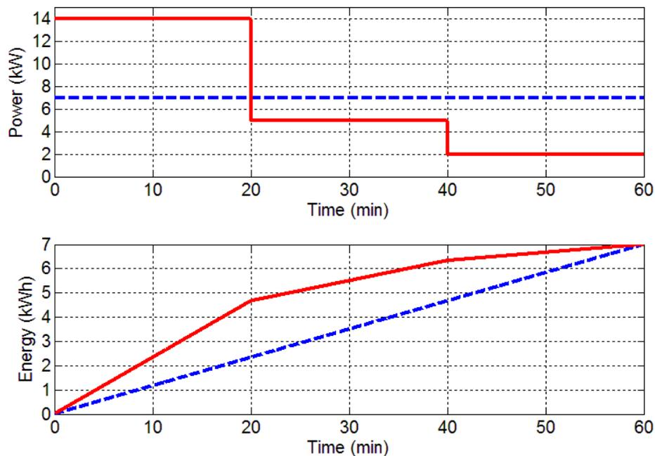
*Fig. 7. Example of the operation principle of the control system during a measuring period in a demand tariff context*
