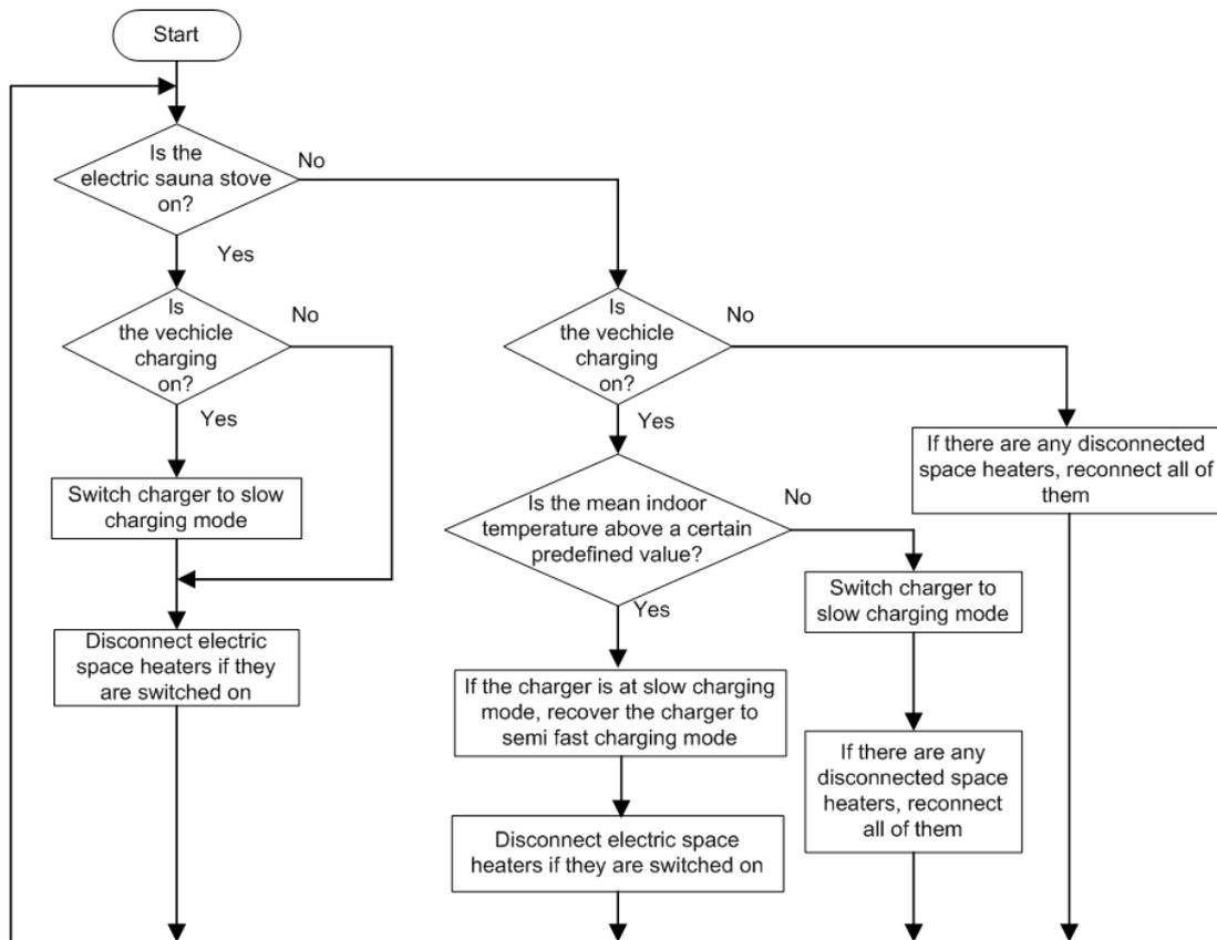
Fig. 4. A peak load management algorithm.
