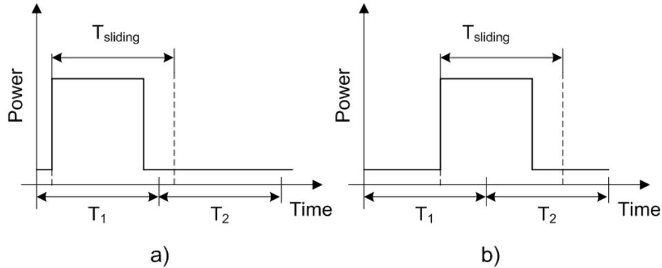
**Fig. 1.** The differences between the predefined and sliding measurement periods.
