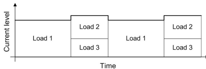
Fig. 5. Simplified principle of an alternation method based on pulse-like switching
