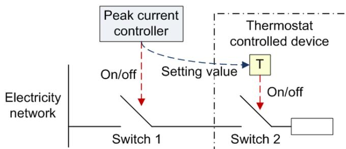
**Fig. 8.** Operation of a thermostat controlled device in peak load controller system.
