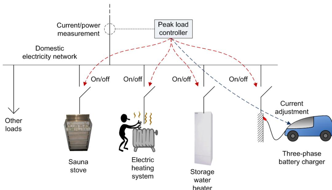
**Fig. 3.** The simplified principle of a peak load management system of for example detached houses.
