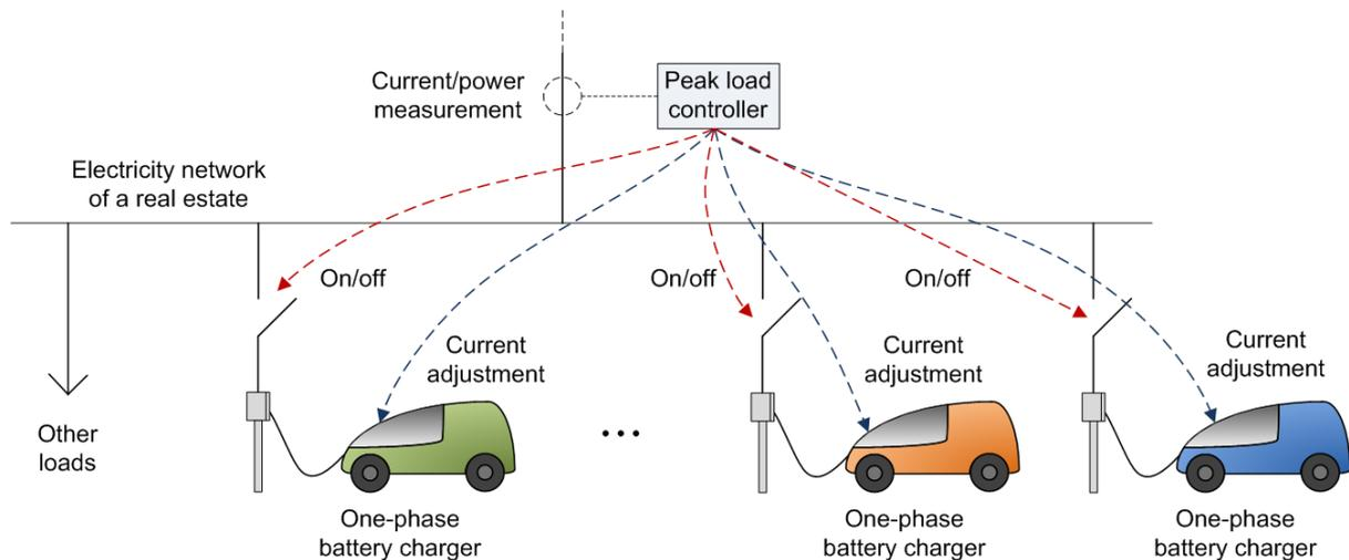
**Fig. 8.** The simplified principle of a peak load management system of parking places including many chargers.
