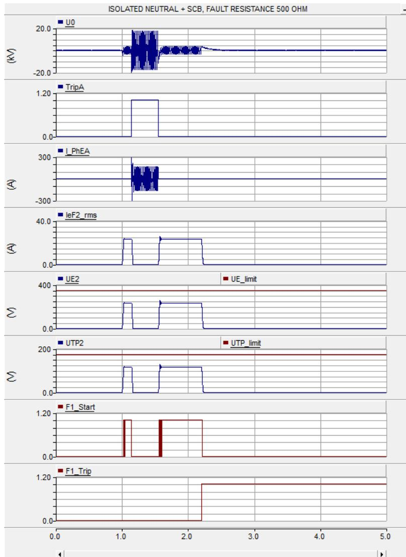
Figure 8. Applying SCB with neutral isolated system when fault resistance was 500 Ω.
