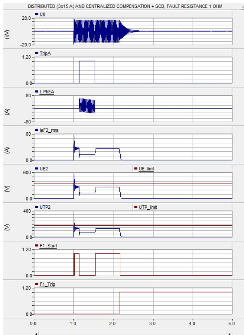
Figure 13. Applying SCB with distributed (3x15A) and centralized compensation when fault resistance was 1 Ω.
