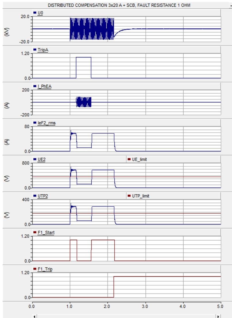
Figure 11. Applying SCB with distributed compensation 3x20 A when fault resistance was 1 Ω.
