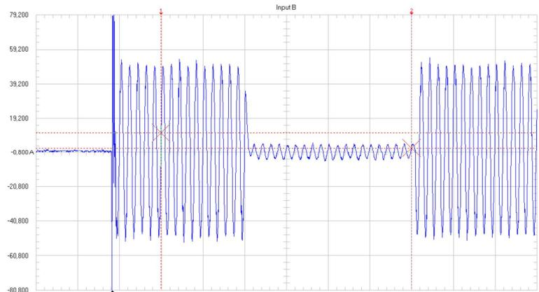
Figure 3. Fault current at the fault location with the phase earthing system.
