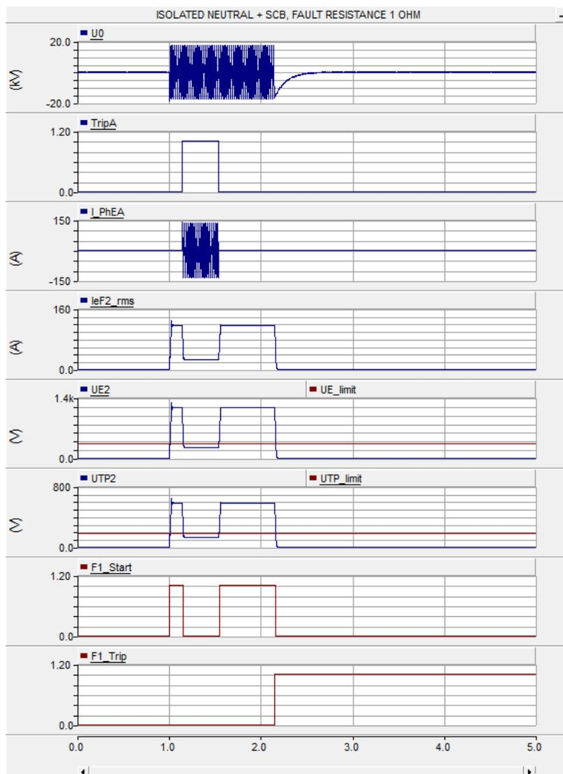
Figure 7. Applying SCB with neutral isolated system when fault resistance was 1 Ω.
