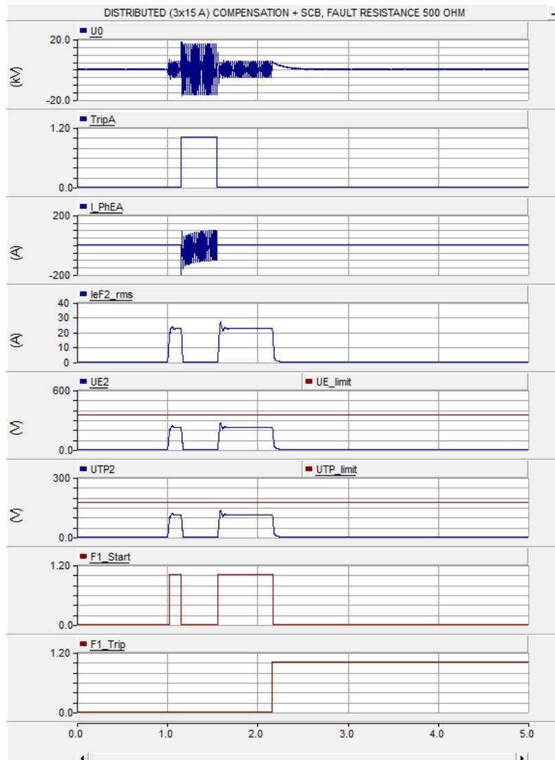
Figure 10. Applying SCB with distributed compensation 3x15 A when fault resistance was 500 Ω.
