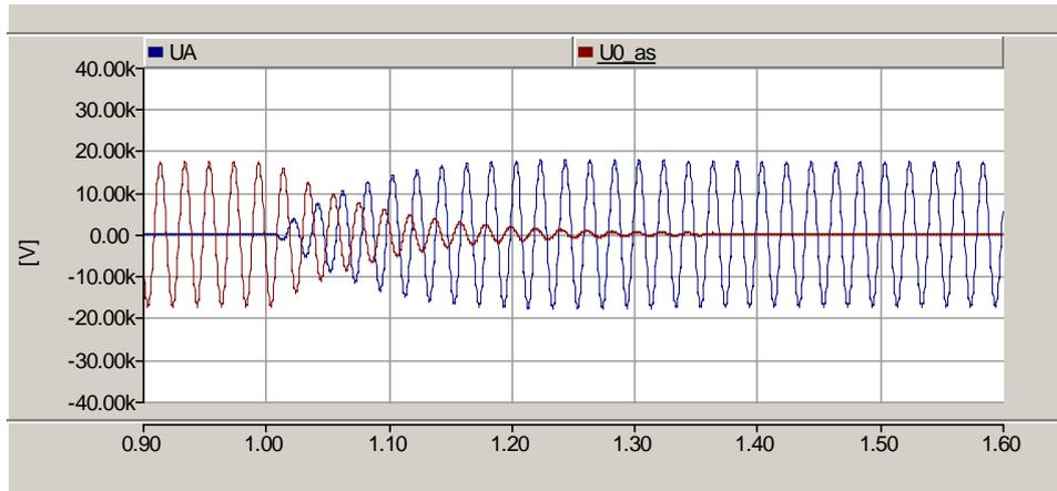
**Figure 5.** Recovery voltage ( $U_A$ ) and neutral voltage ( $U_0$ ) after earth fault arc extinction in neutral compensated network.
