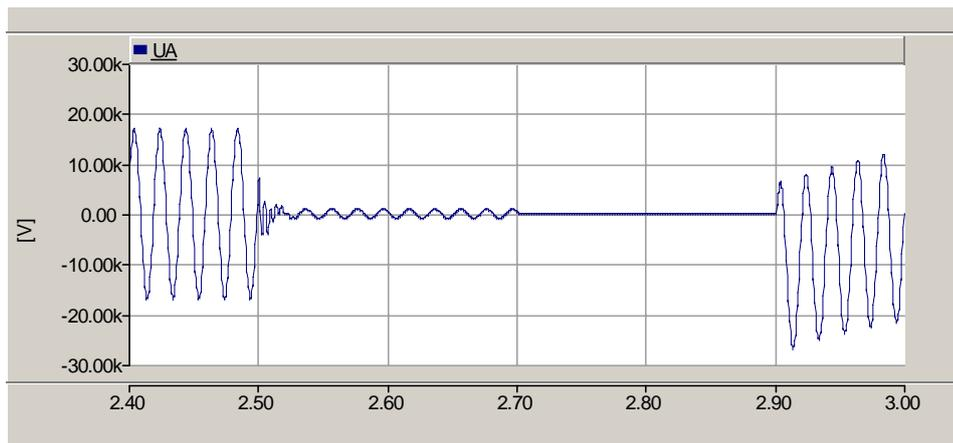
**Figure 6.** Recovery voltage ( $U_A$ ) after earth fault arc extinction when phase earthing is applied with neutral isolated network.
