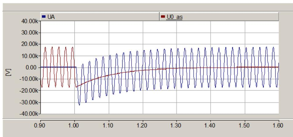
**Figure 4.** Recovery voltage ( $U_A$ ) and neutral voltage ( $U_0$ ) after earth fault arc extinction in neutral isolated network.
