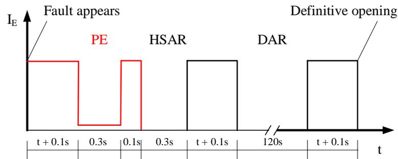
Figure 1. Operation sequence of PE and E/F protection with neutral compensated system.
