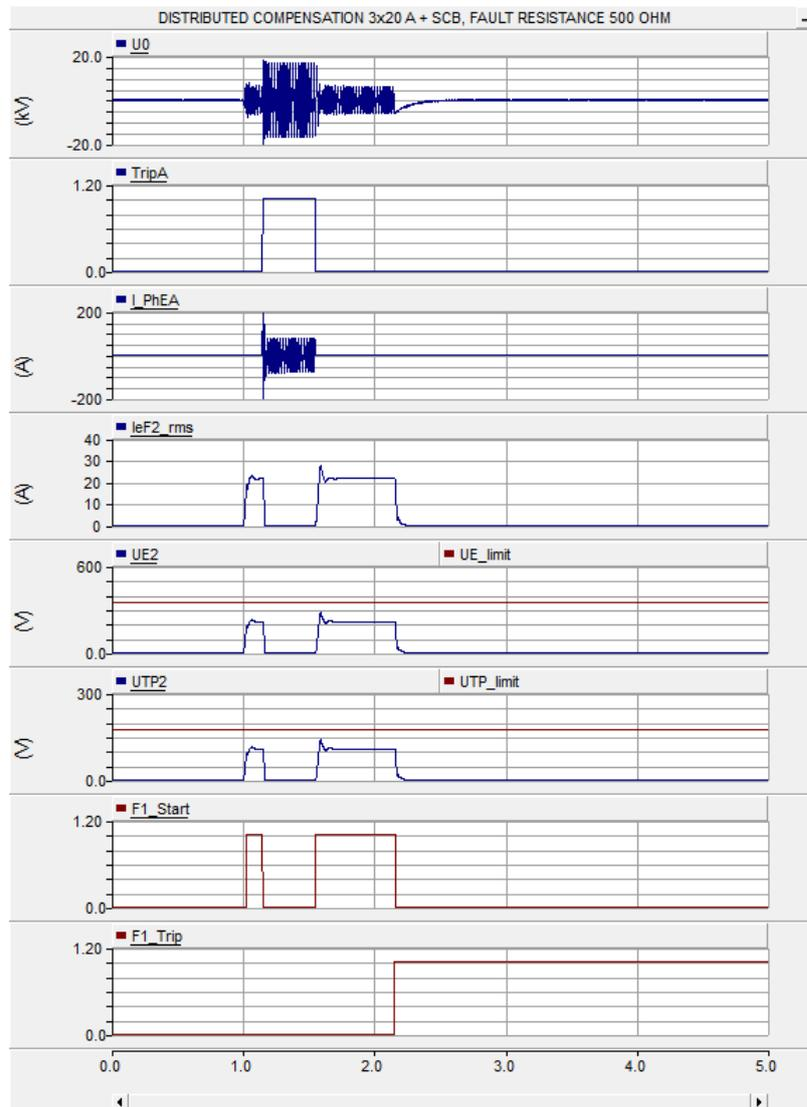
**Figure 12.** Applying SCB with distributed compensation 3x20 A when fault resistance was 500  $\Omega$ .
