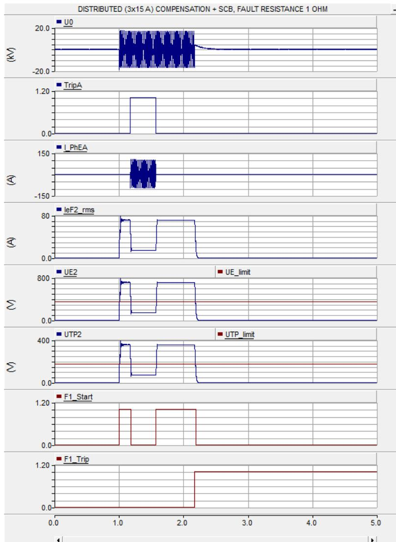
Figure 9. Applying SCB with distributed compensation 3x15A when fault resistance was 1 Ω.
