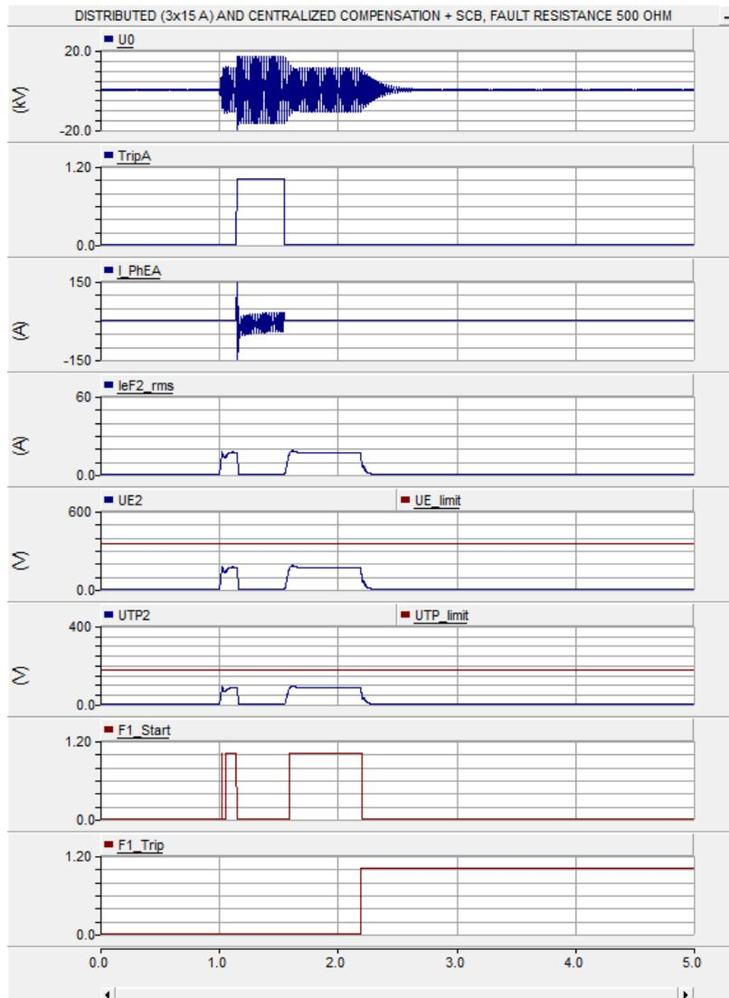
**Figure 14.** Applying SCB with distributed (3x15 A) and centralized compensation when fault resistance was 500 Ω.
