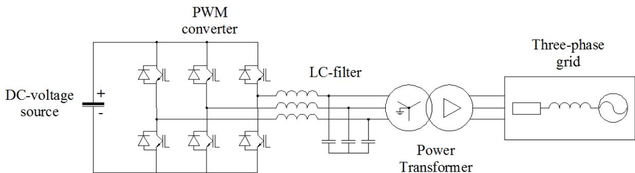
Figure 2.1 The structure of the wind power converter model
