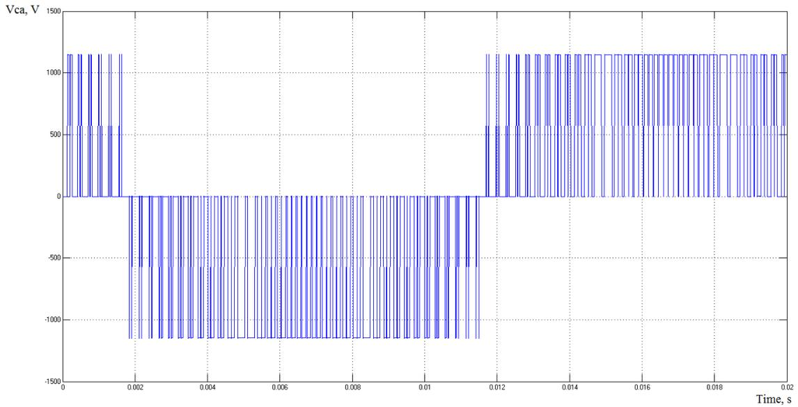
Figure 2.4 The line-to-line voltage in PWM inverter
