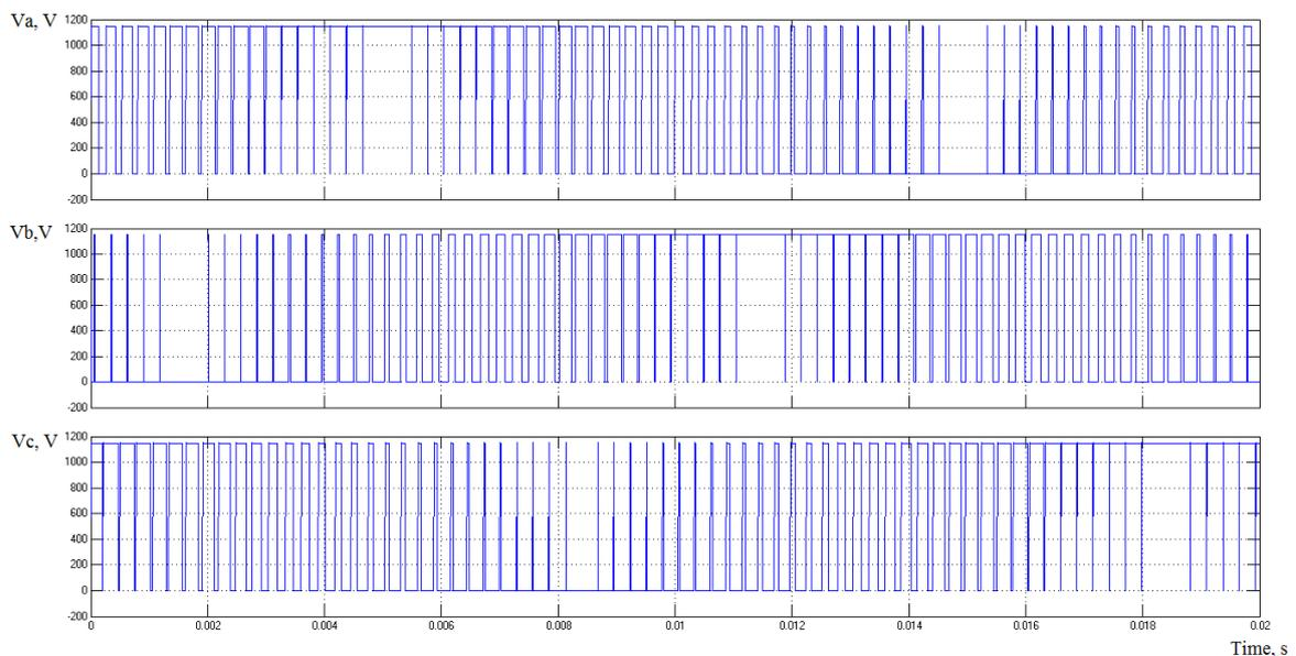
Figure 2.3 Output phase voltages of PWM inverter
