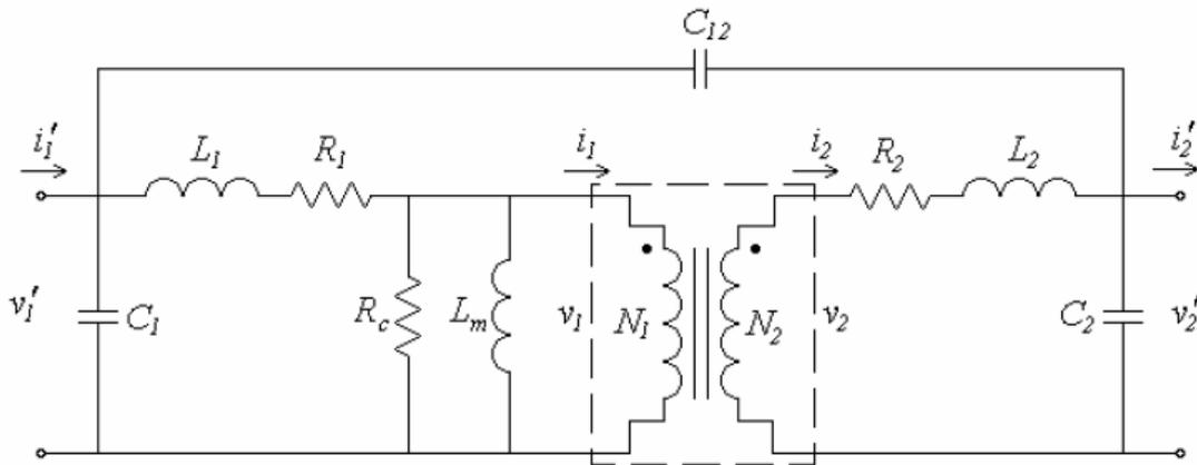
Figure 2.10 equivalent circuit of a broadband transformer (Wong 2004)
