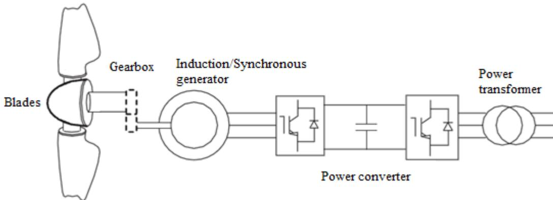
Figure 1.1. The scheme of variable-speed FRC wind turbine (Anaya-Lara et al. 2009)
