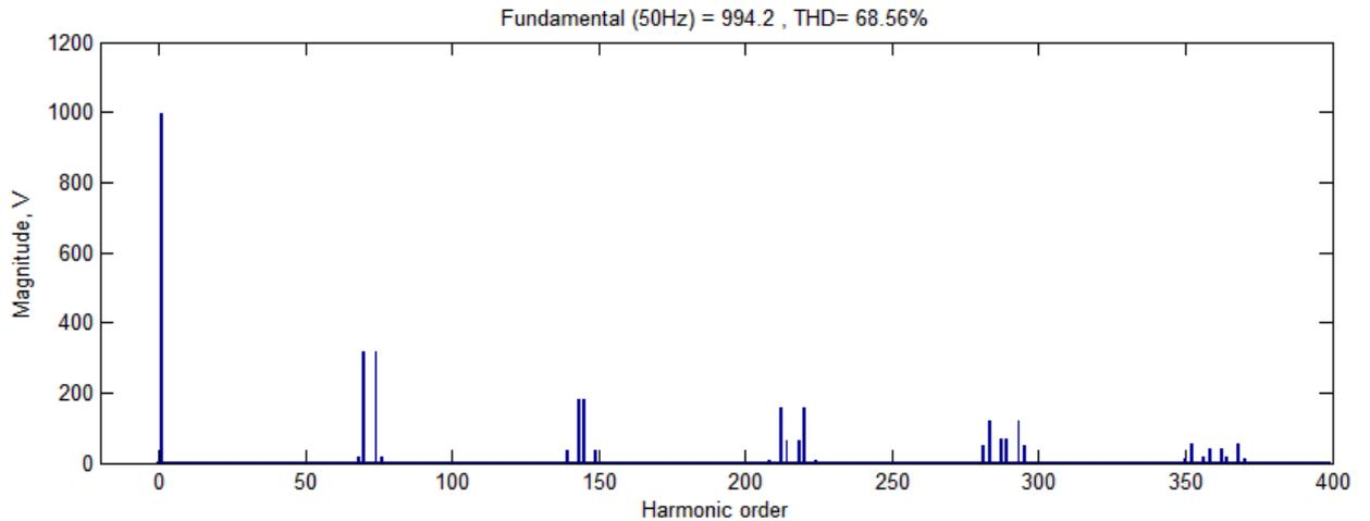
Figure 2.5 FFT analysis of line-to-line voltage of PWM inverter
