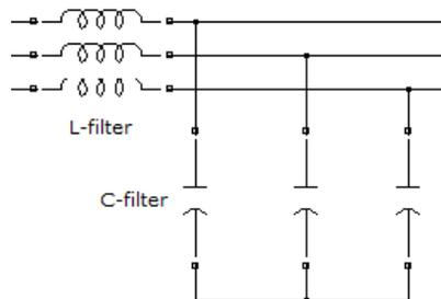
Figure 2.6. Model of LC-filter in Simulink
