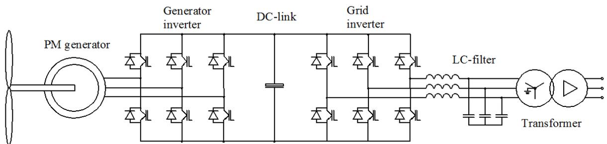
Figure 1.2 Electrical part of variable-speed wind turbine
