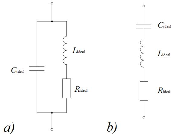
Figure 2.7. a) Model of a real inductor b) model of a real capacitor
