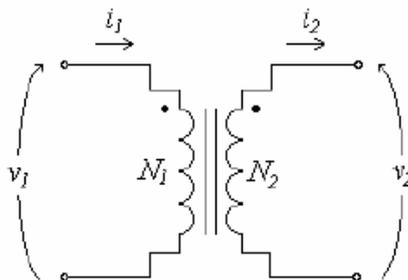
Figure 2.8 Electrical model of an ideal transformer (Wong 2004)
