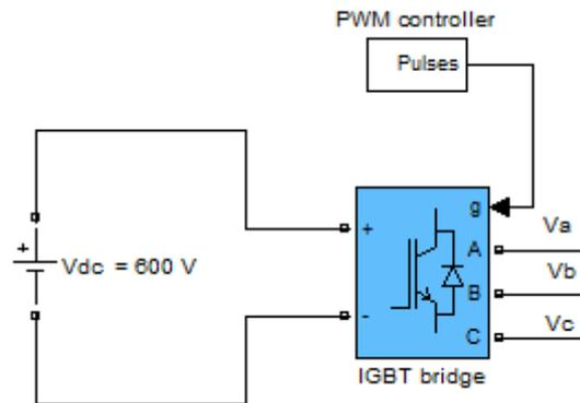
Figure 2.2 The model of PWM inverter in Matlab
