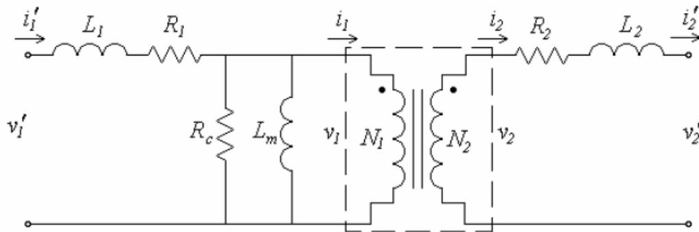
Figure 2.9. Electrical model of a real transformer (Wong 2004)
