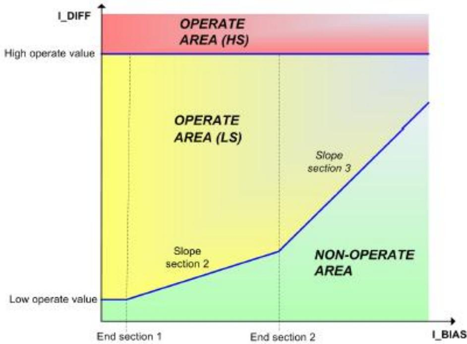
Fig 7. Operating principle of differential protection
