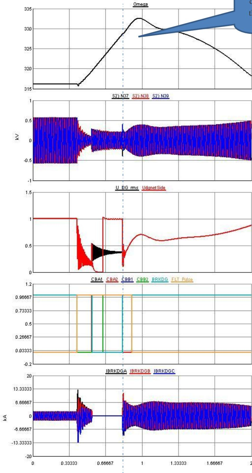
Fig. 5. 1.8MVA induction generator, original weak network, pf0.98ind, Rr=0.0062pu
