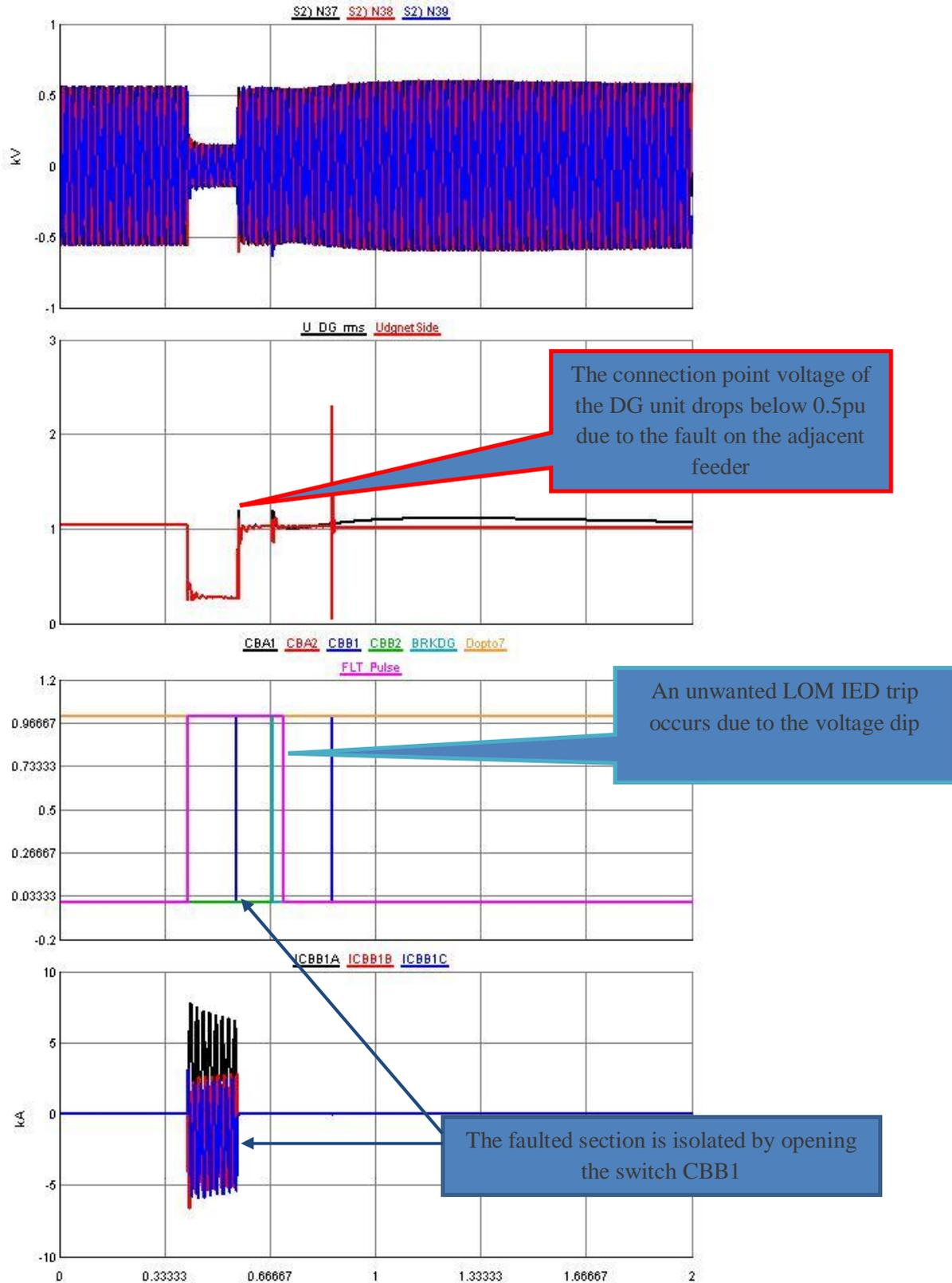
Fig 3. No inter-IED communication, a three phase short circuit in the beginning of feeder B
