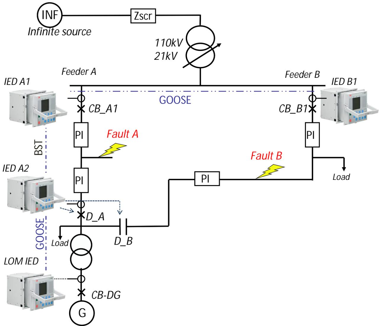
Fig. 1. The network model used in radial network configuration studies
