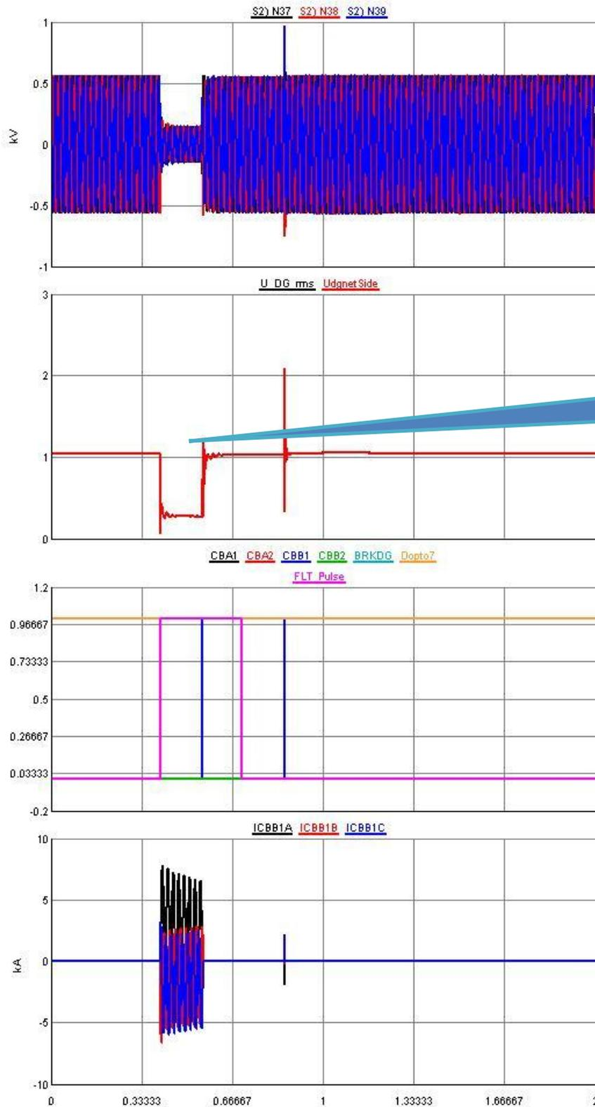
Fig. 4. With inter-IED communication, a three phase short circuit in the beginning of feeder B, a block command from IED03 blocks the UV protection of the DG relay.
