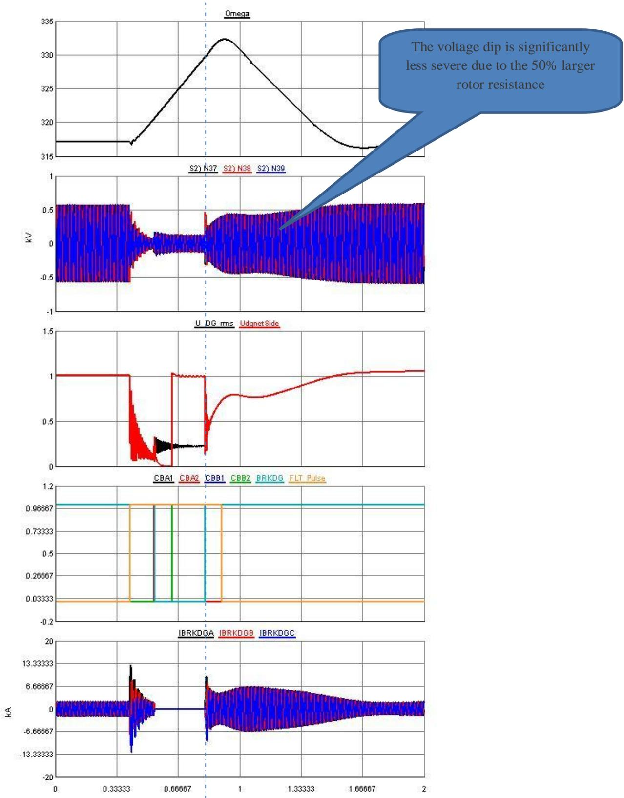
Fig. 6. 1.8MVA induction generator, original weak network, pf0.98ind, Rr=0.0093pu
