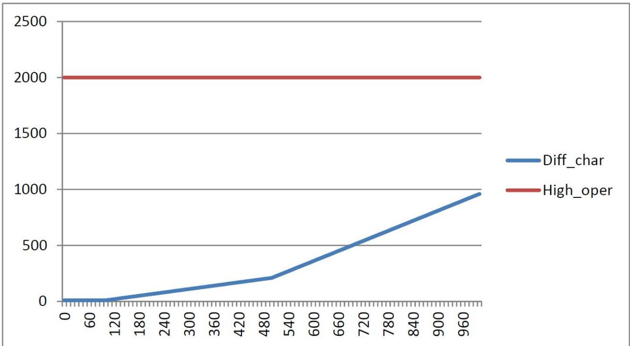
Fig. 8. Operating characteristics of the utilized differential protection function
