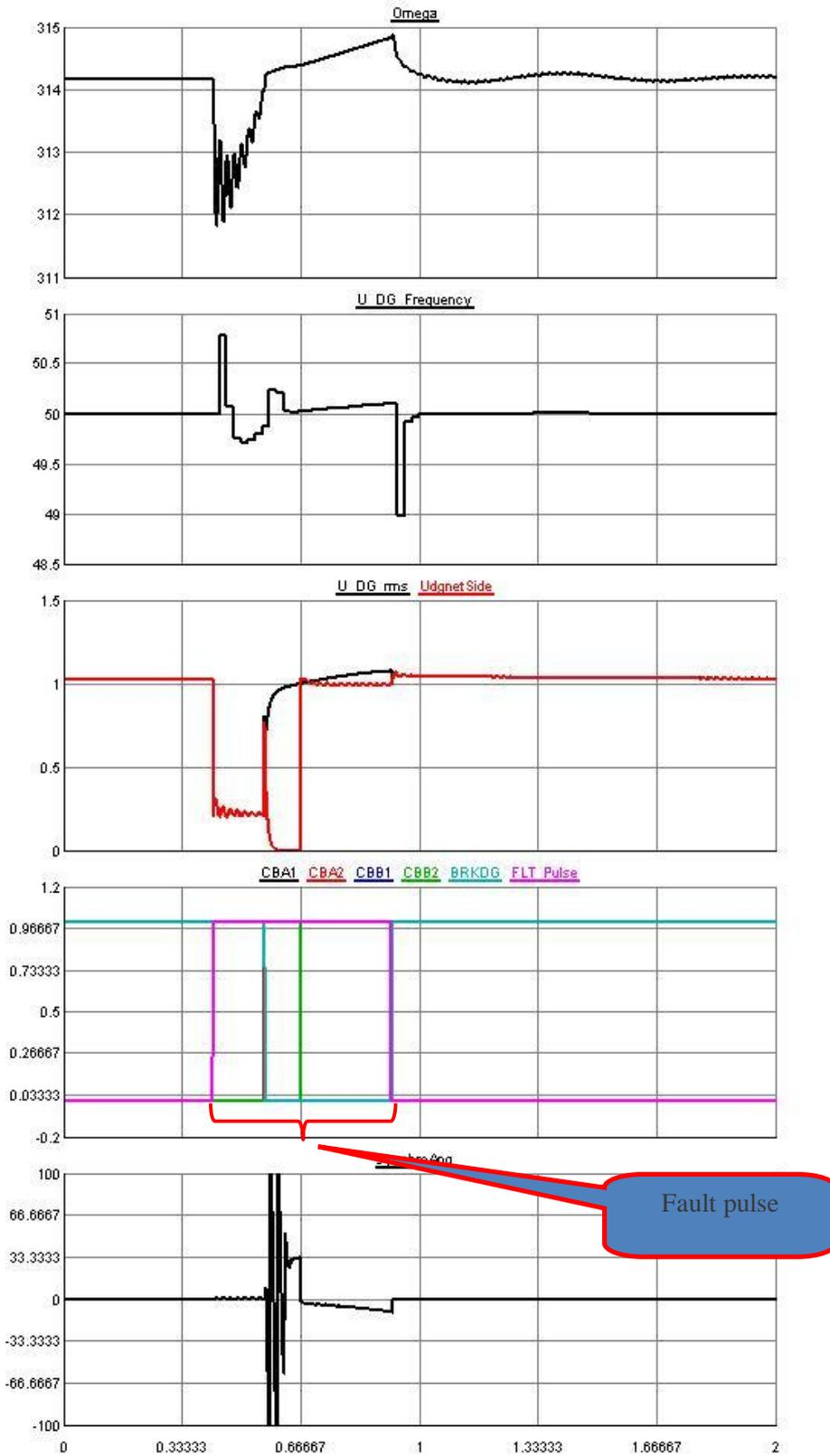
Fig. 2. Chosen graphs from the SG1600MVA, H=2, Tm0.43pu case presented in table III.
