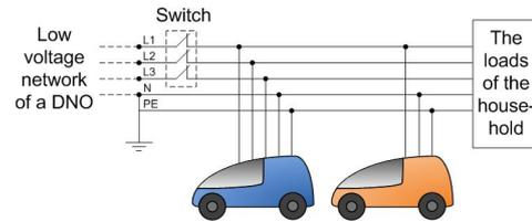
Fig. 2. Realization of the vehicle-to-home service.
