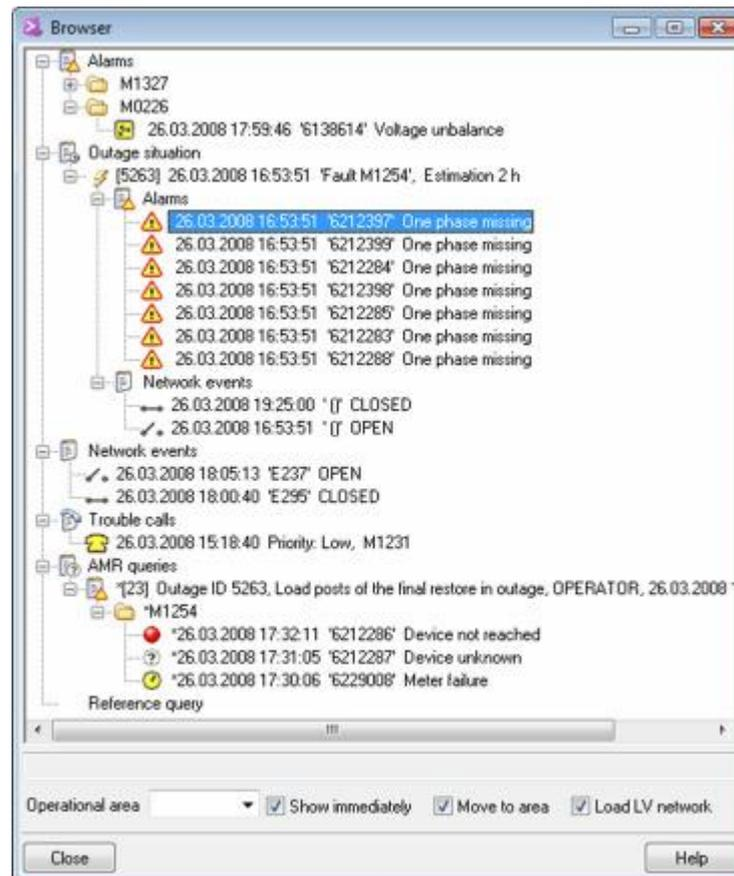
**Figure 1.** Tree structure tool for managing operational data in Tekla DMS
