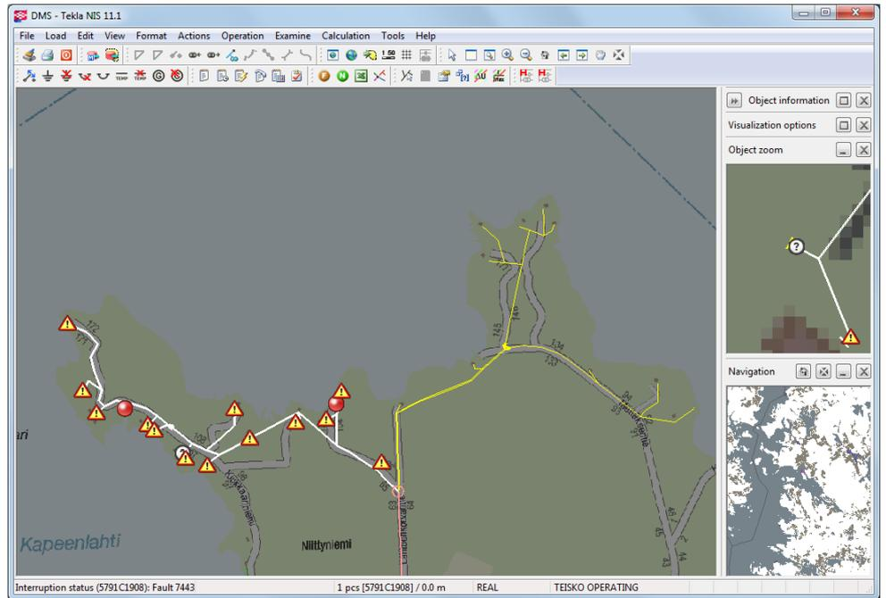
**Figure 2.** Visualization of AMR alarm data on the network map in Tekla DMS
