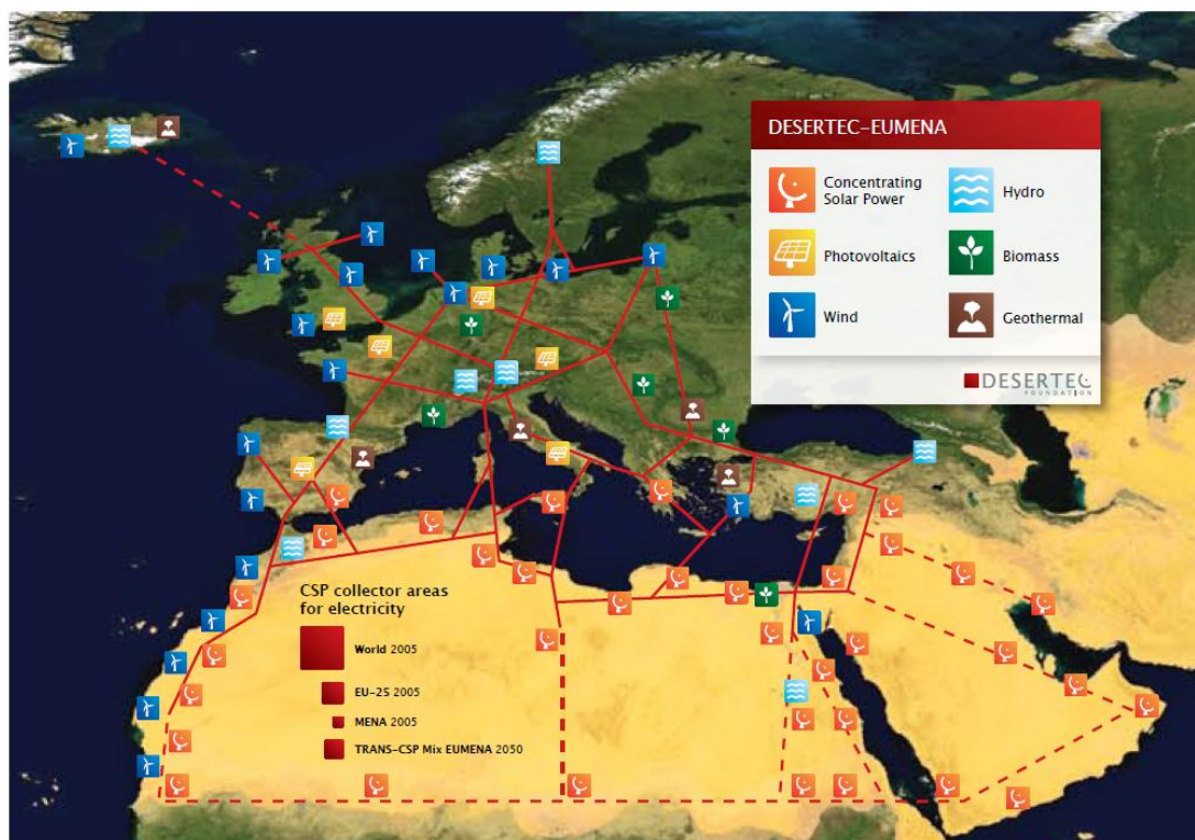
Figure 36. Concept of a “EUMENA Supergrid” based on HVDC power transmission as “Electricity Highways” to complement the conventional AC electricity grid, as developed by TREC in 2003. The symbols for power sources and lines are only sketching typical locations. Reprinted from Desertec Foundation 2009.
