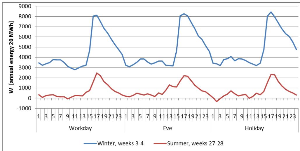
Figure 2. Resulting heating profile when load profile 601 of a one family house (5 MWh per year), with no electric heat and no sauna, is subtracted from load profile 110, a direct electric heated one family house (25 MWh per year), during selected winter and summer weeks and according to weekday type. Load profiles 110 and 601 are here based on index series. NB. The days here are traditional power utility day 07:00-07:00.
