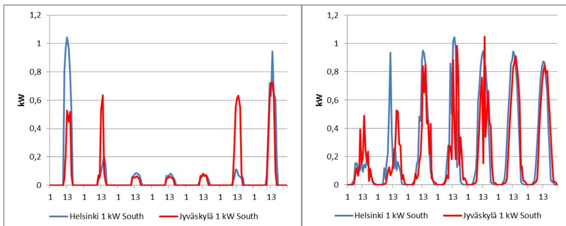
Figure 10. Calculated PV production in Helsinki and Jyväskylä 23.-29.1.2014 to the left and 1.-7.7.2014 to the right based on measured solar radiations. The PV panel is angled directly south.
