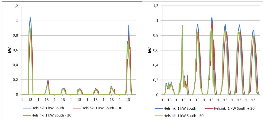
Figure 9. Calculated PV production in Helsinki 23.-29.1.2014 to the left and 1.-7.7.2014 to the right based on measured solar radiations. The PV panel is angled directly or  $\pm 30^\circ$  south.
