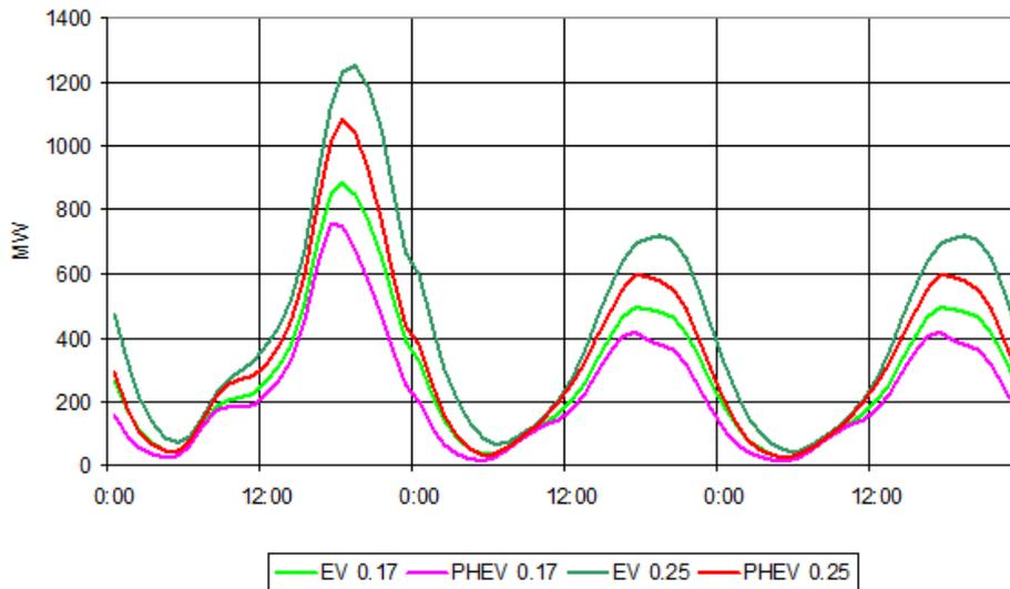
Figure 7. Daily charging profile for one million electric vehicles, of different types, assuming charging begins as soon as cars are plugged in. 0.17 refers to a consumption of 0.17 kWh/km of full EV sedan and 0.25 kWh/km for a sport utility type of full EV. PHEVs use less electricity as they run partly on gasoline. Source: Koreneff et al. 2009
