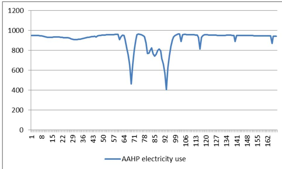
Figure 5. AAHP electricity use as an auxiliary heat source in a non-electrically heated house for the same seven days as shown in Figure 3. Data source: SGEM WT3.6 (FP1), see Laitinen et al. 2011.
