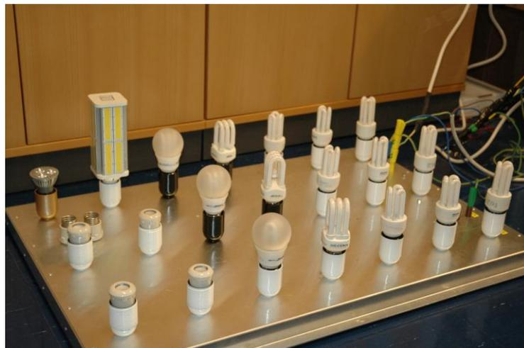
**Fig. 9 Load model based on CFL and LED lamps built at TUT**
