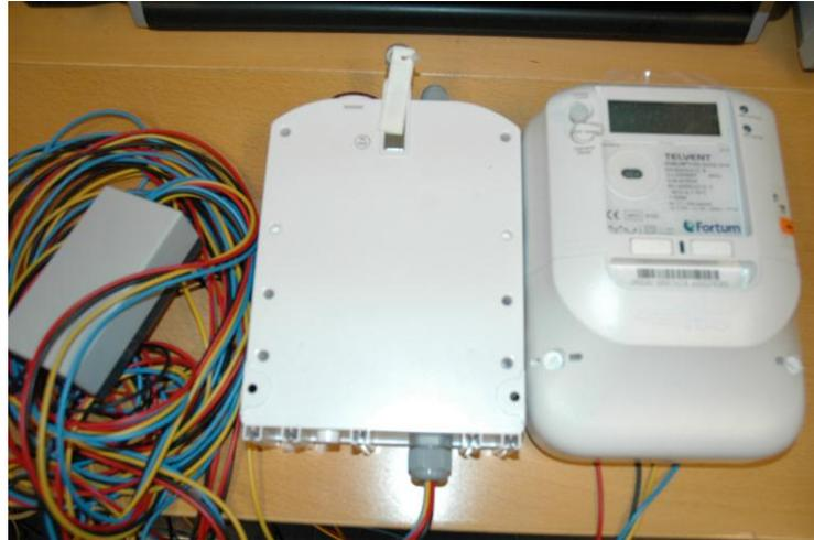
**Fig. 8 Smart meter and concentrator setup**
