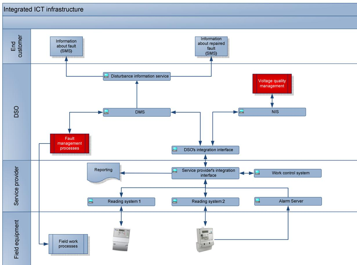
**Figure 2.** A system map related to smart fault management of the low voltage network.
