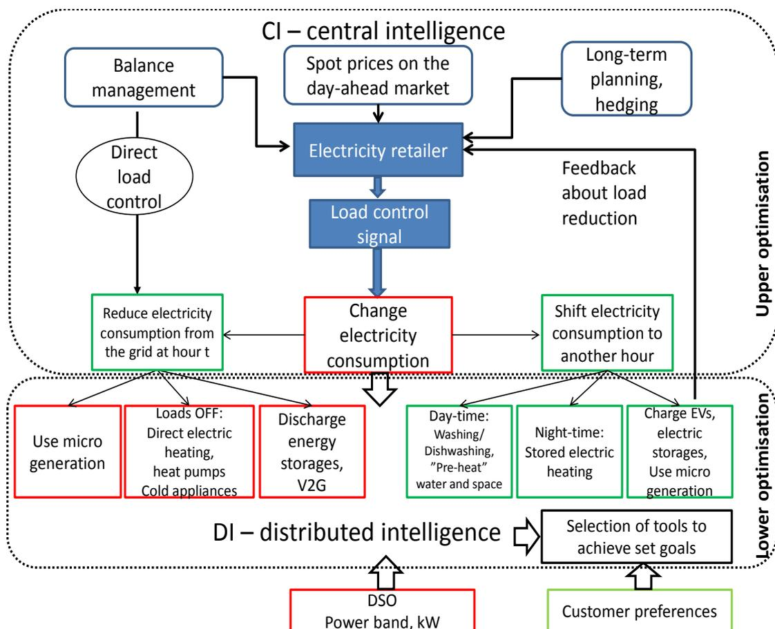
Figure 3.2. Operational model for load control in INCA.
