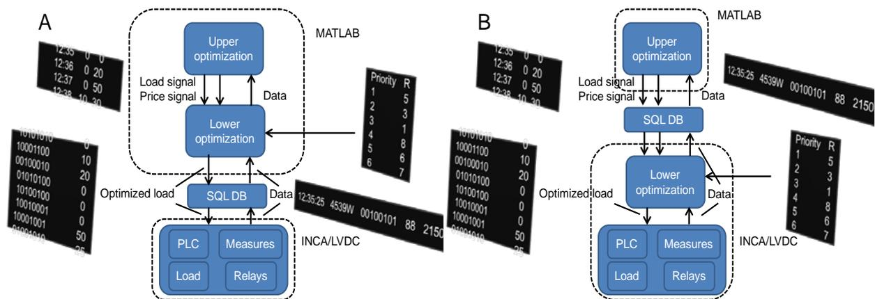
Figure 4.3. Information structure of INCA laboratory pilot at first phase (A) and second phase (B).
