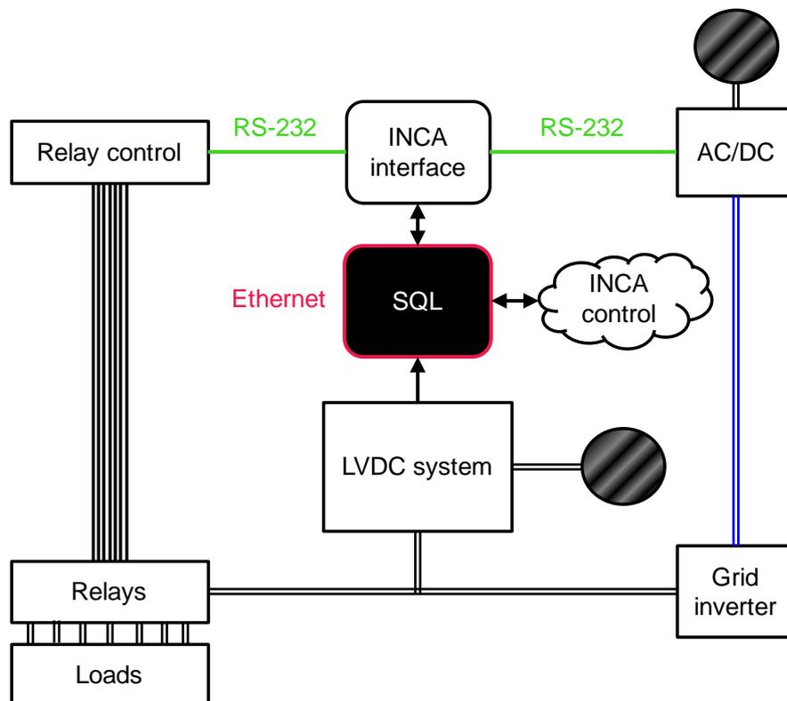
Figure 4.1. Technical structure of the INCA laboratory setup.
