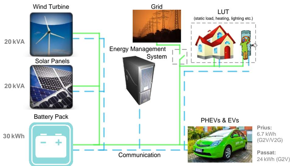
Figure 1.2. Basic concept of the Green Campus Smart Grid.
