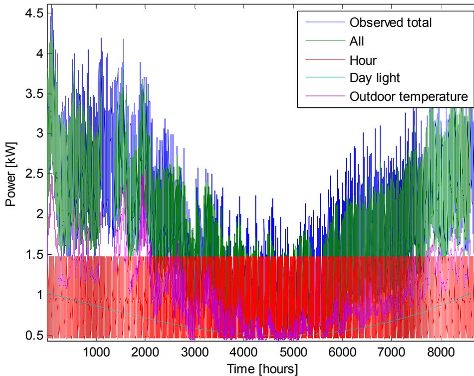
**Figure 2.** Sub loads modelled using the SVR model (modified from Niska 2013, IEEE ISSNIP 2013).
