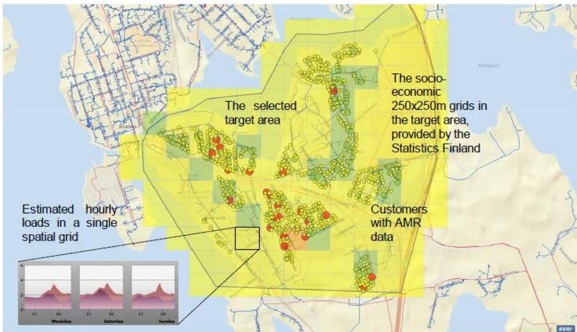
**Figure 3.** Spatial load modelling concept based on the spatial grids (modified from Niska et al. 2013, CIRED 2013).
