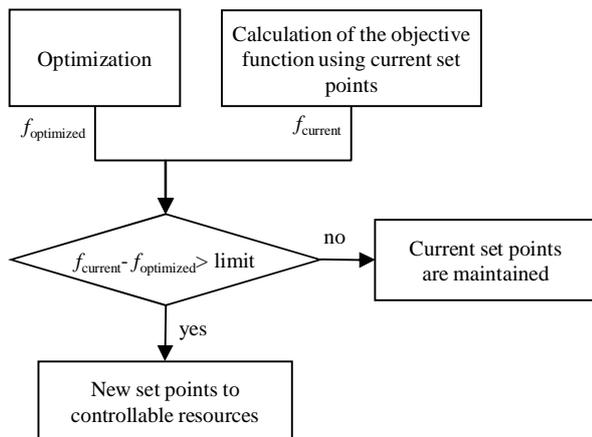
Figure 9. The algorithm part that checks whether to execute the changes suggested by the optimization algorithm.
