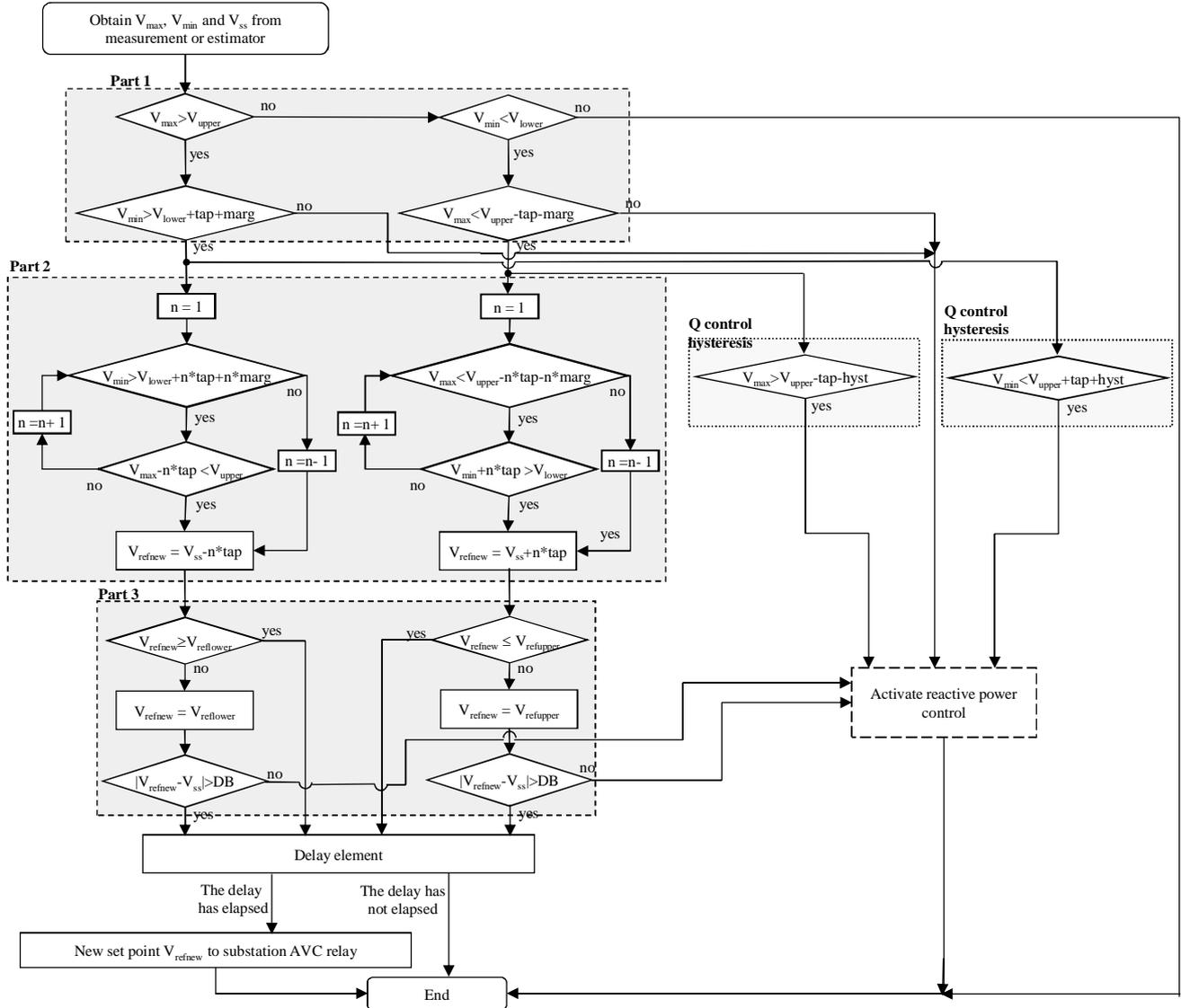
Figure 2. The flow chart of basic substation voltage control.
