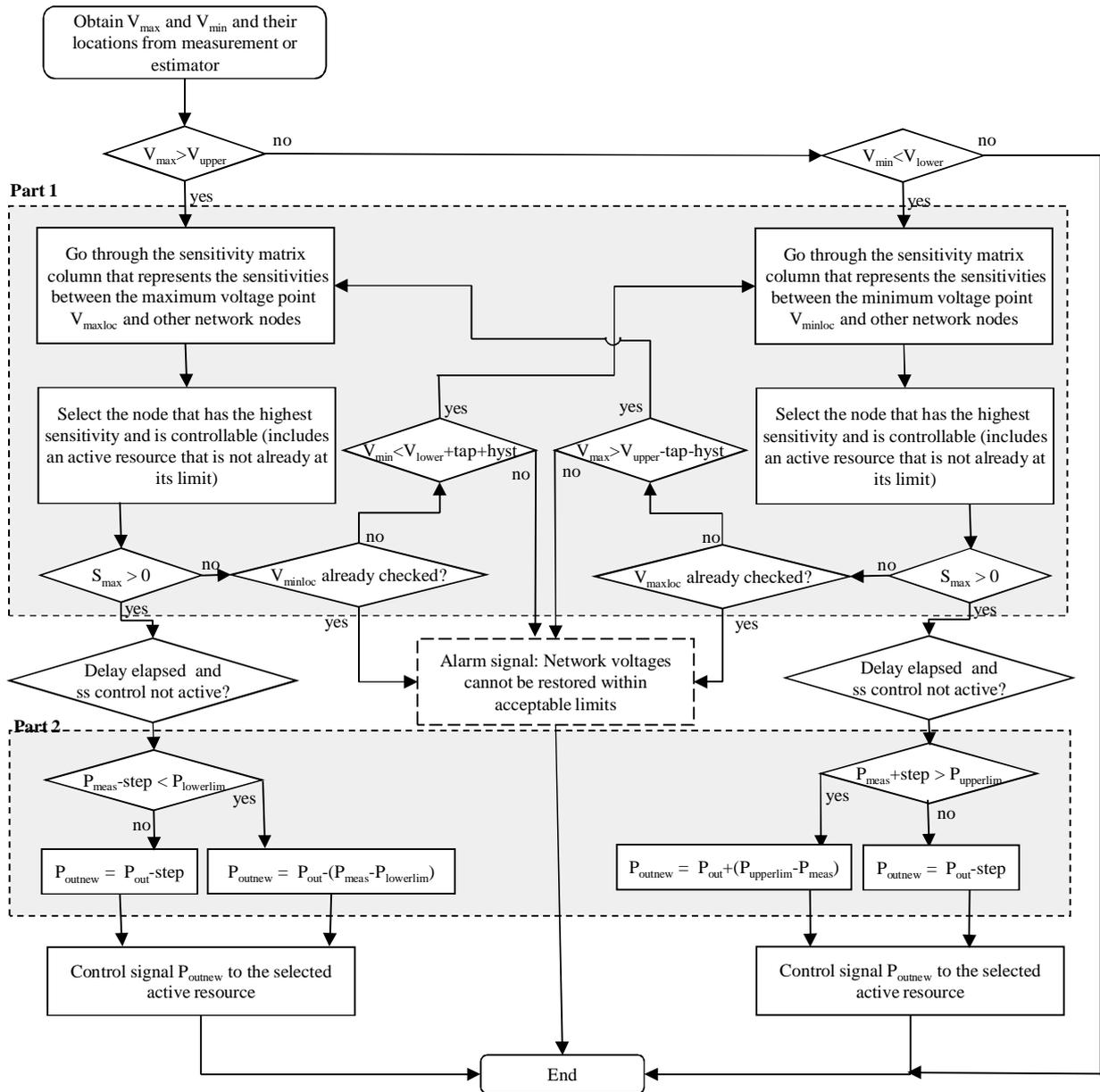
Figure 4. The flow chart of basic real power control.
