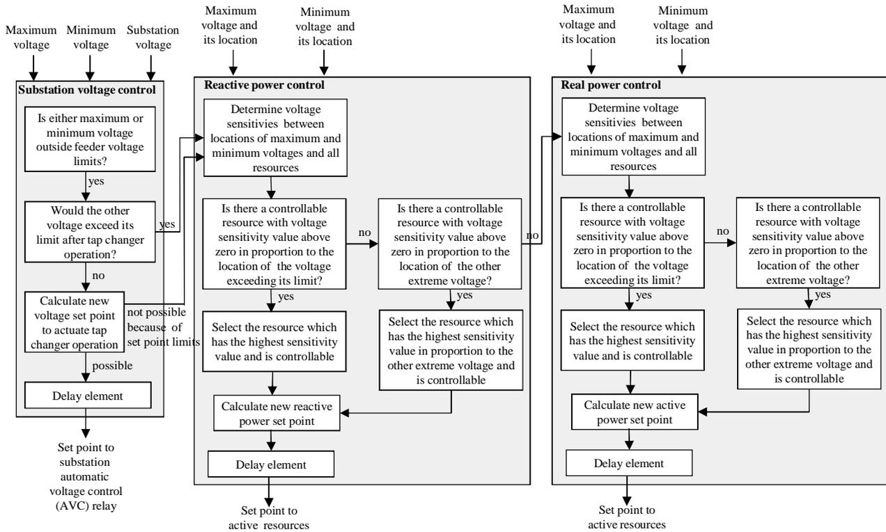
Figure 1. The operational principle of basic control.
