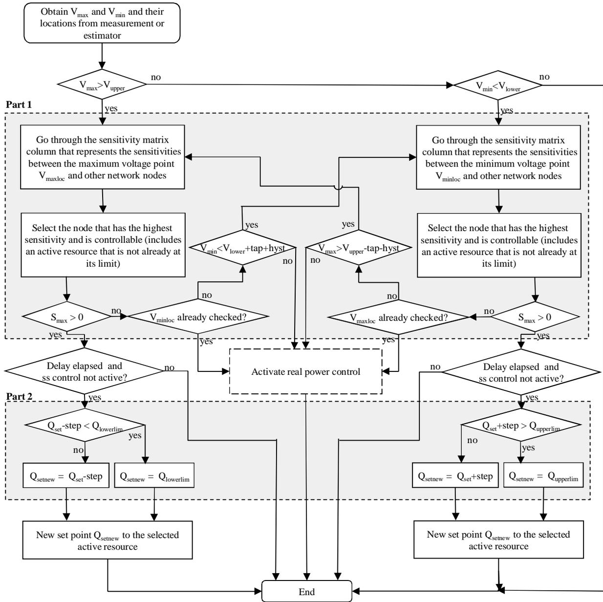
Figure 3. The flow chart of basic reactive power control.
