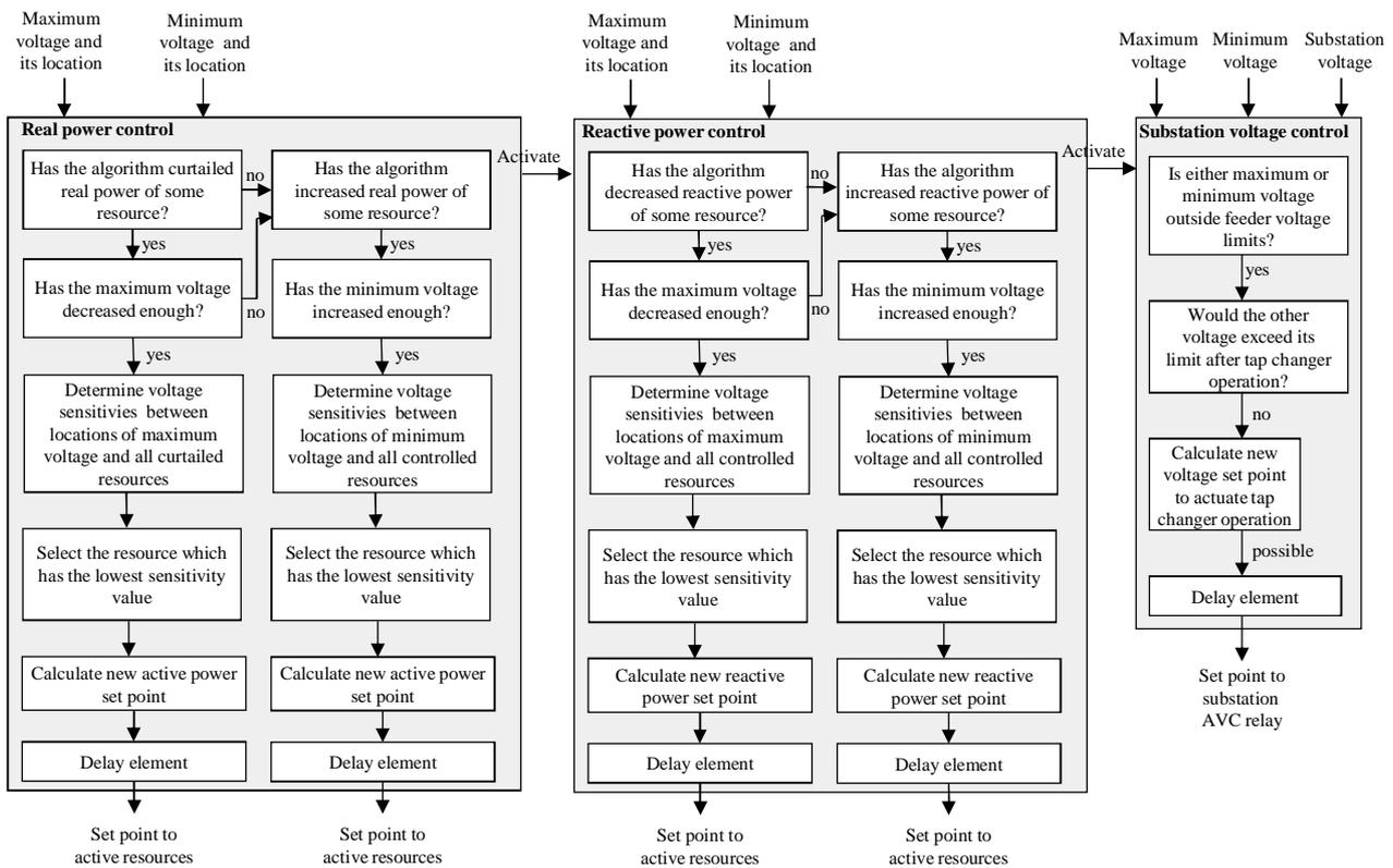
Figure 5. The operational principle of restoring control.
