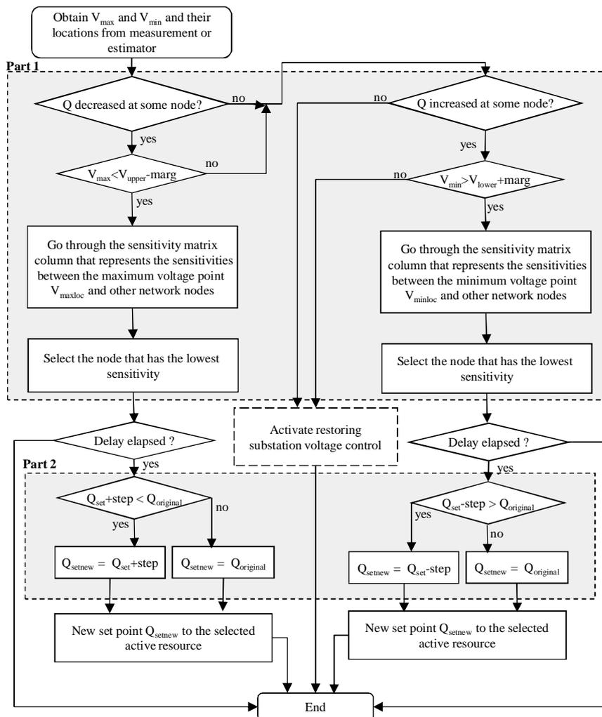
Figure 7. The flow chart of restoring reactive power control.
