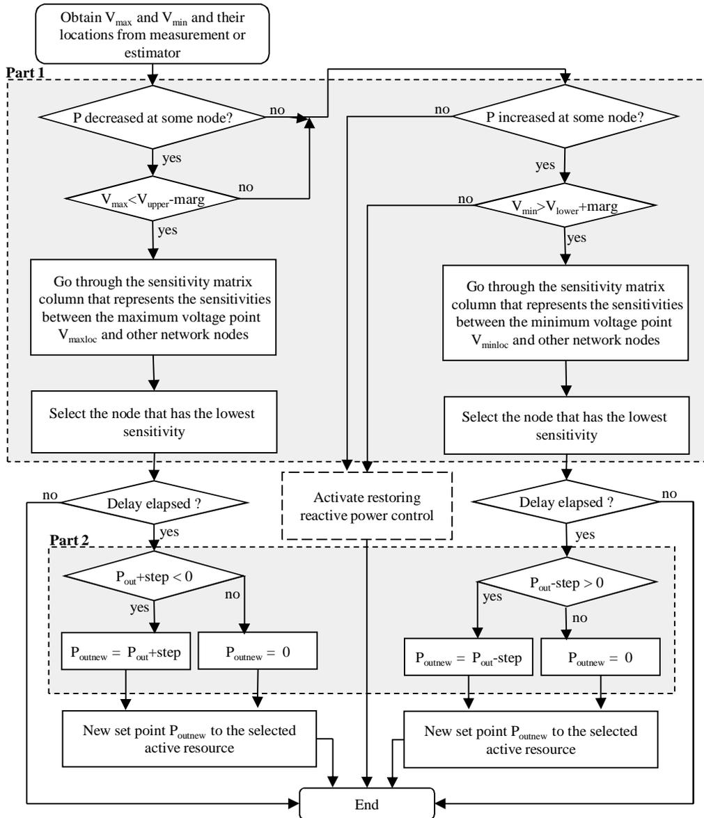
Figure 6. The flow chart of restoring real power control.
