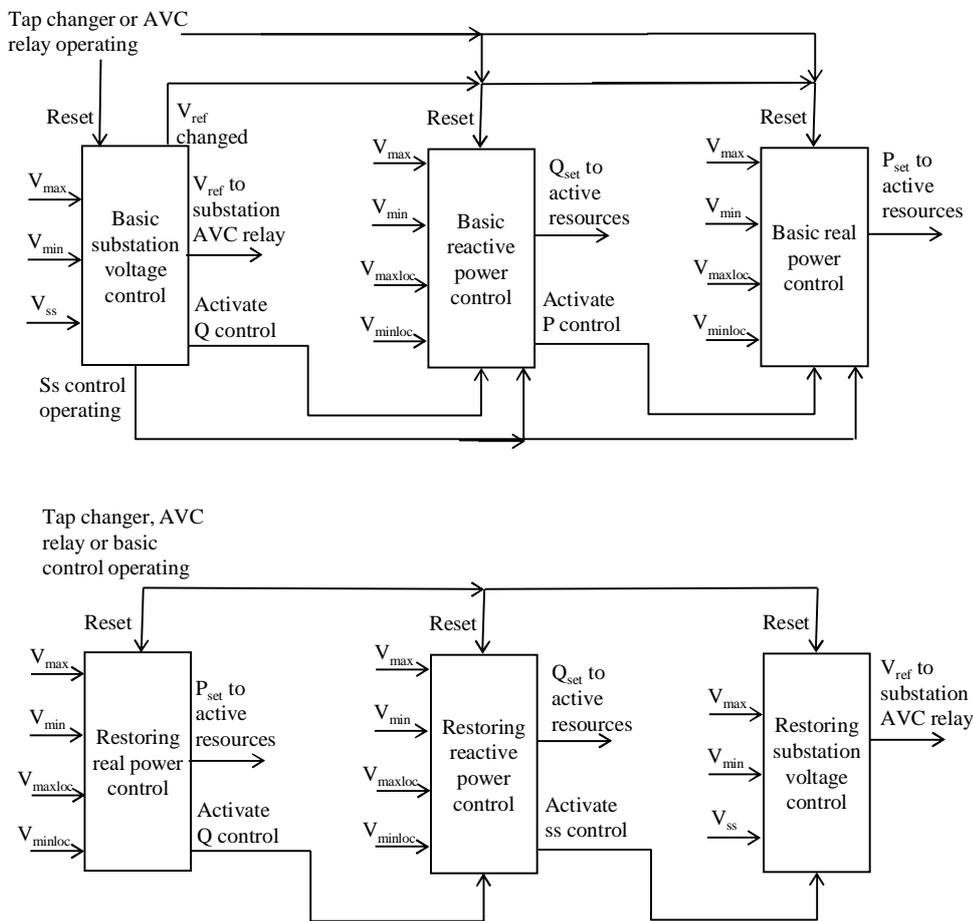
Figure 8. The inputs and outputs and the connections between control blocks.
