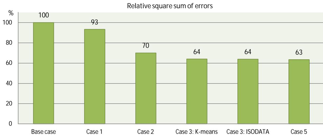
**Figure 1.** Comparison between different load profiling methods when modelling residential customers [2].
