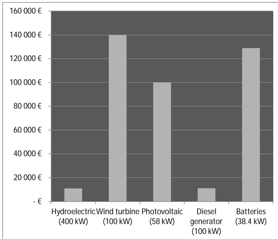
**Figure 7. Optional investment costs of a microgrid capable of generating about 100 kW.**
