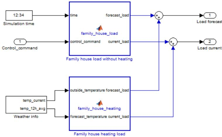
Figure 12. Load block of a single-family house
