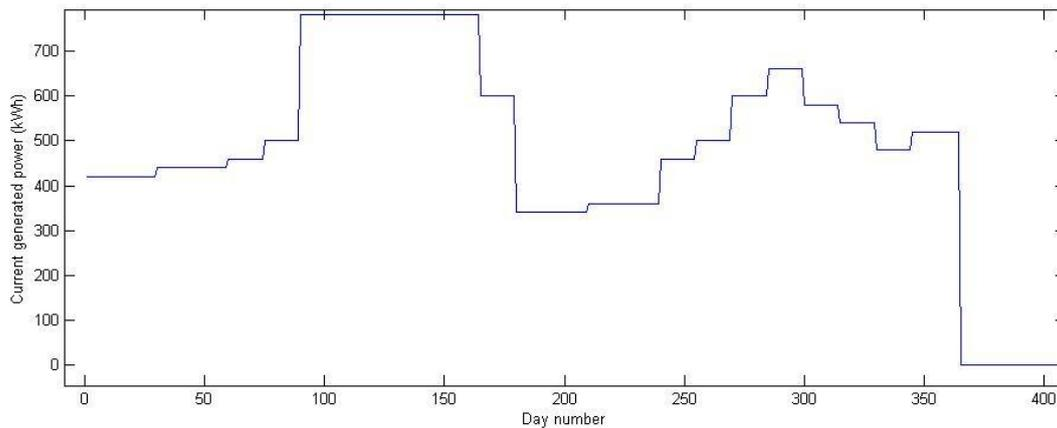
**Figure 10. Generated power of a single hydroelectric power generator for a year with default parameters**
