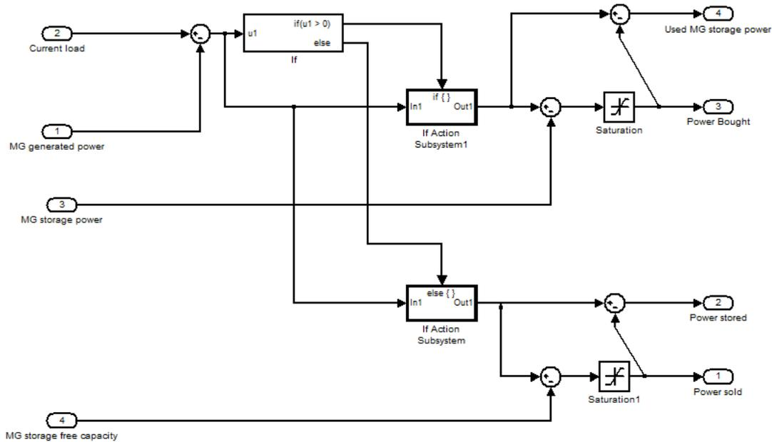
Figure 3. Power Distribution block
