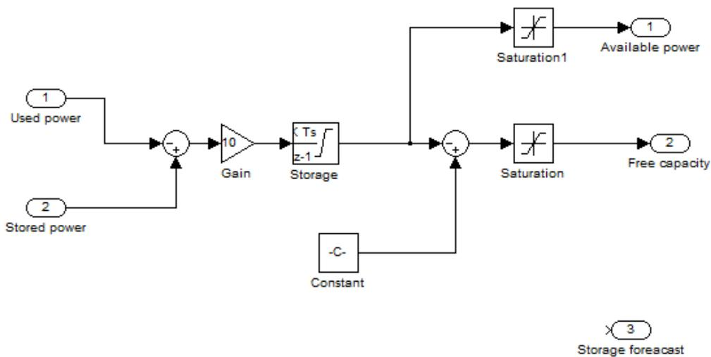
Figure 6. Simulation model for storage components
