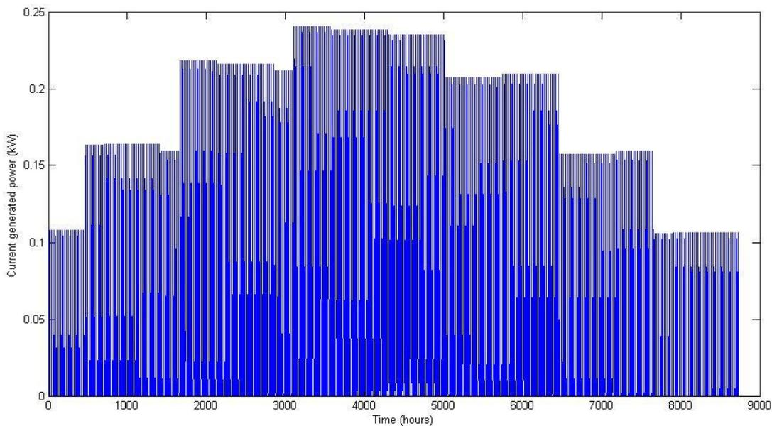
**Figure 9. Hourly generated power of a single Photovoltaic power generator for a year with default parameters**
