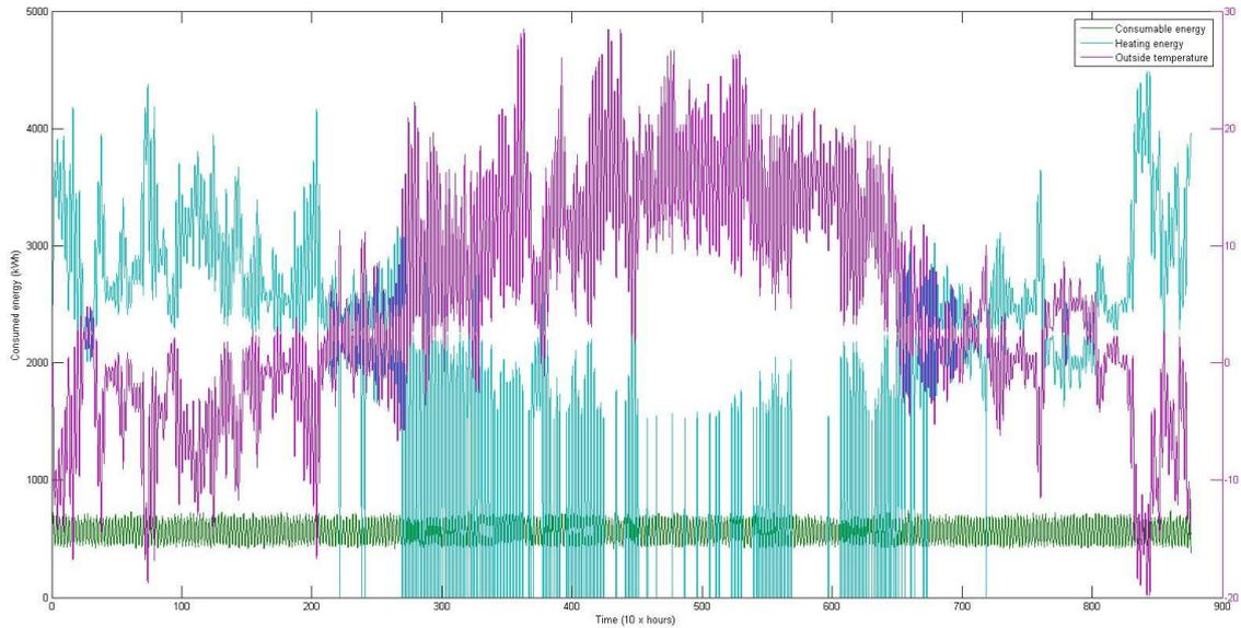
**Figure 13. Yearly 12 hour averaged energy profile of a single family house with default parameters without load control**
