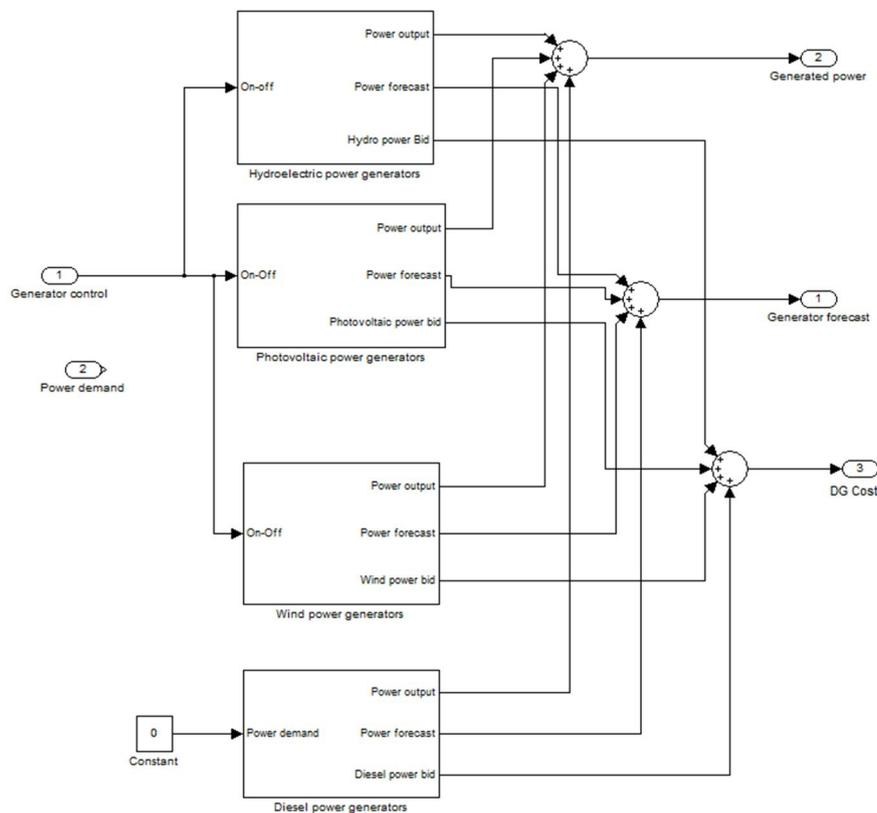
Figure 8. Generator Controller (GC) simulation model
