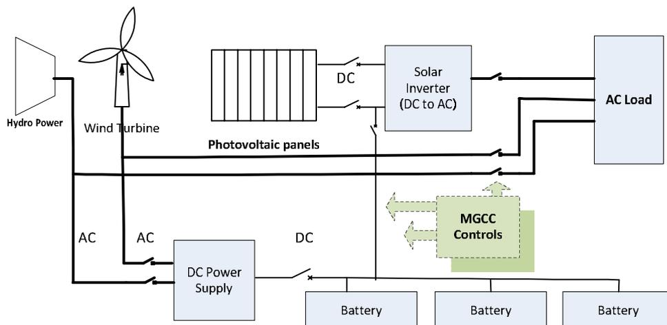
**Figure 5. A simplified view of the main devices required to store the energy which is generated in a microgrid**
