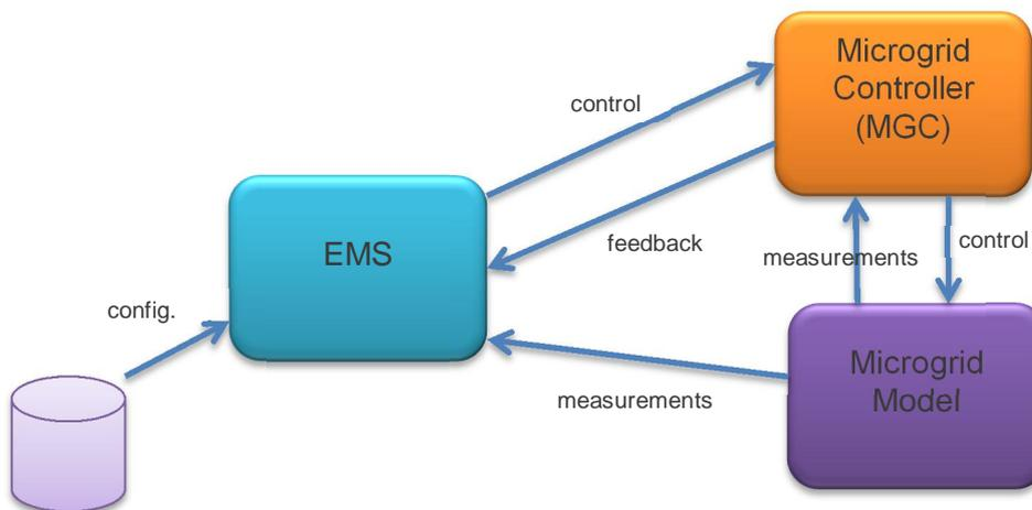
**Figure 3. Data communication between the EMS, the MGC and the microgrid model**
