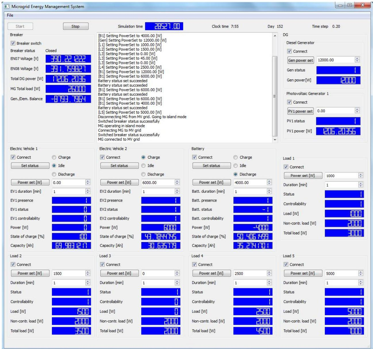
Figure 11. Energy Management System control panel
