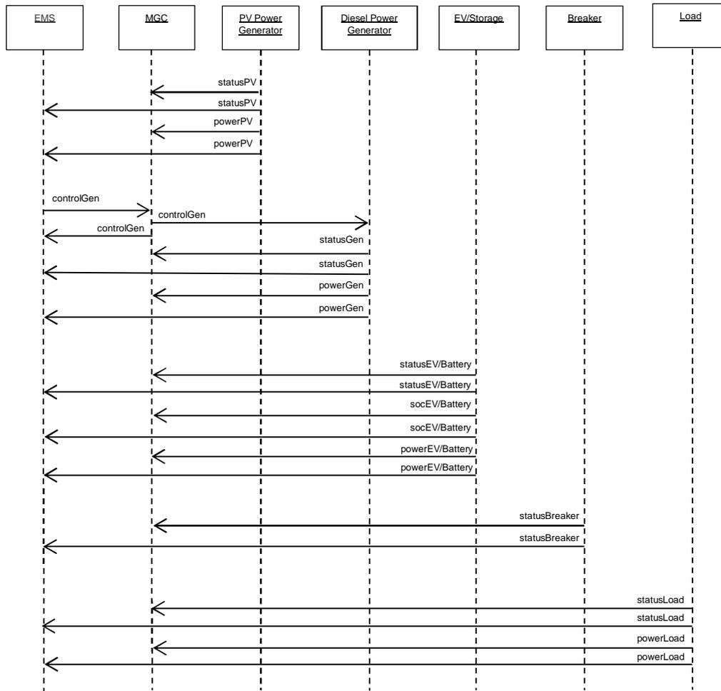
Figure 12. Initialization sequence diagram
