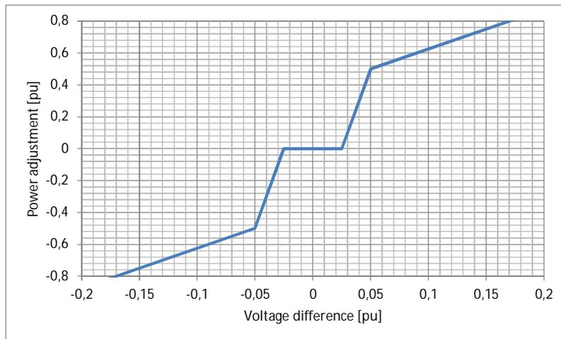
Figure 9. Voltage drop characteristics used in MGC logics
