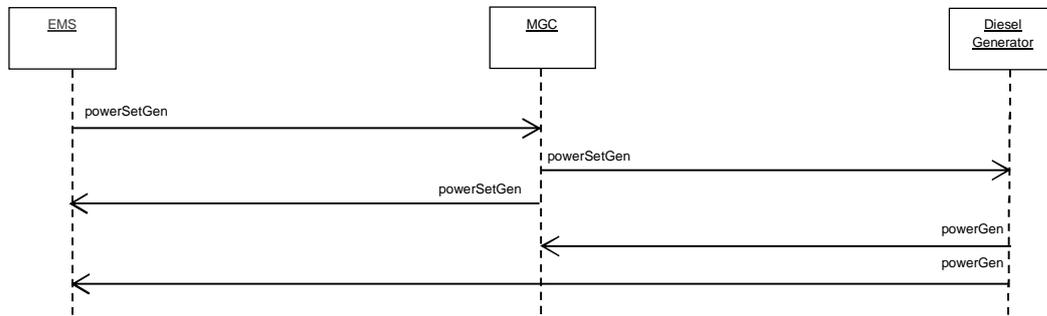
Figure 13. Control of the Diesel Generator
