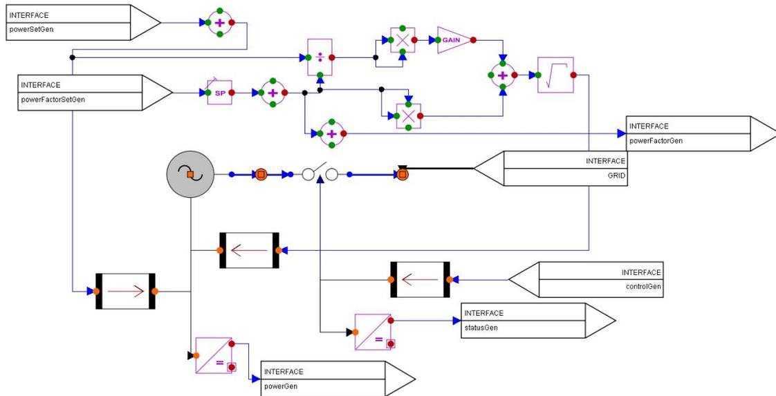
Figure 8. Layout of diesel generator block
