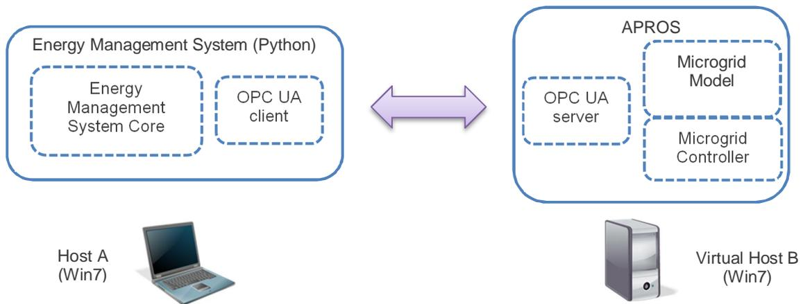
Figure 2. Microgrid Simulation Platform
