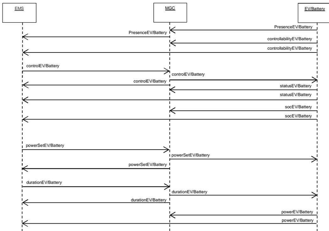
Figure 15. Control of the EV/Battery models
