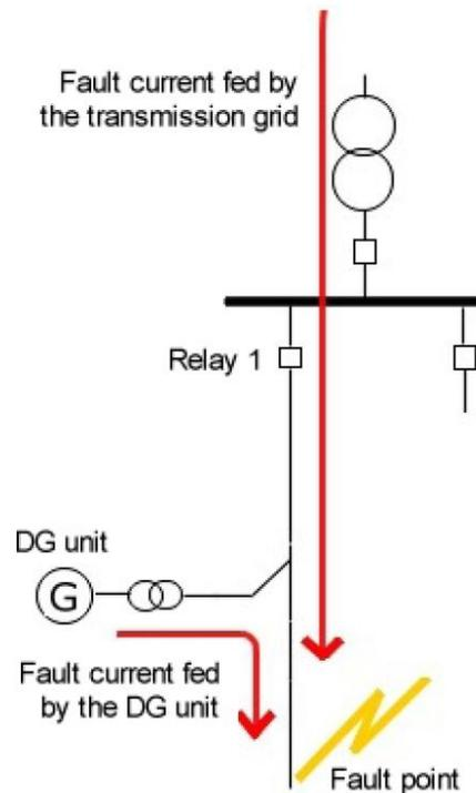
Figure2.1. DG unit causing protection blinding [Mäk05]
