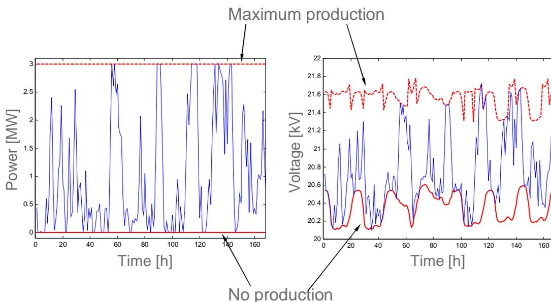
Figure 4.1. Example of hourly time series of power production and connection point voltage.
