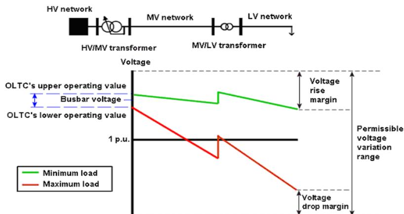
Figure 3.2. Voltage profile of a radial distribution feeder in maximum and minimum loading conditions.
