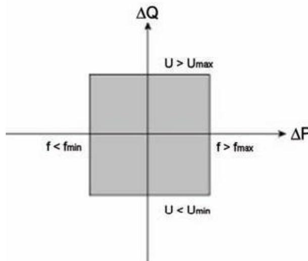
Figure 2.3. Non-detection zone for traditional voltage and frequency protection [Mäk07]
