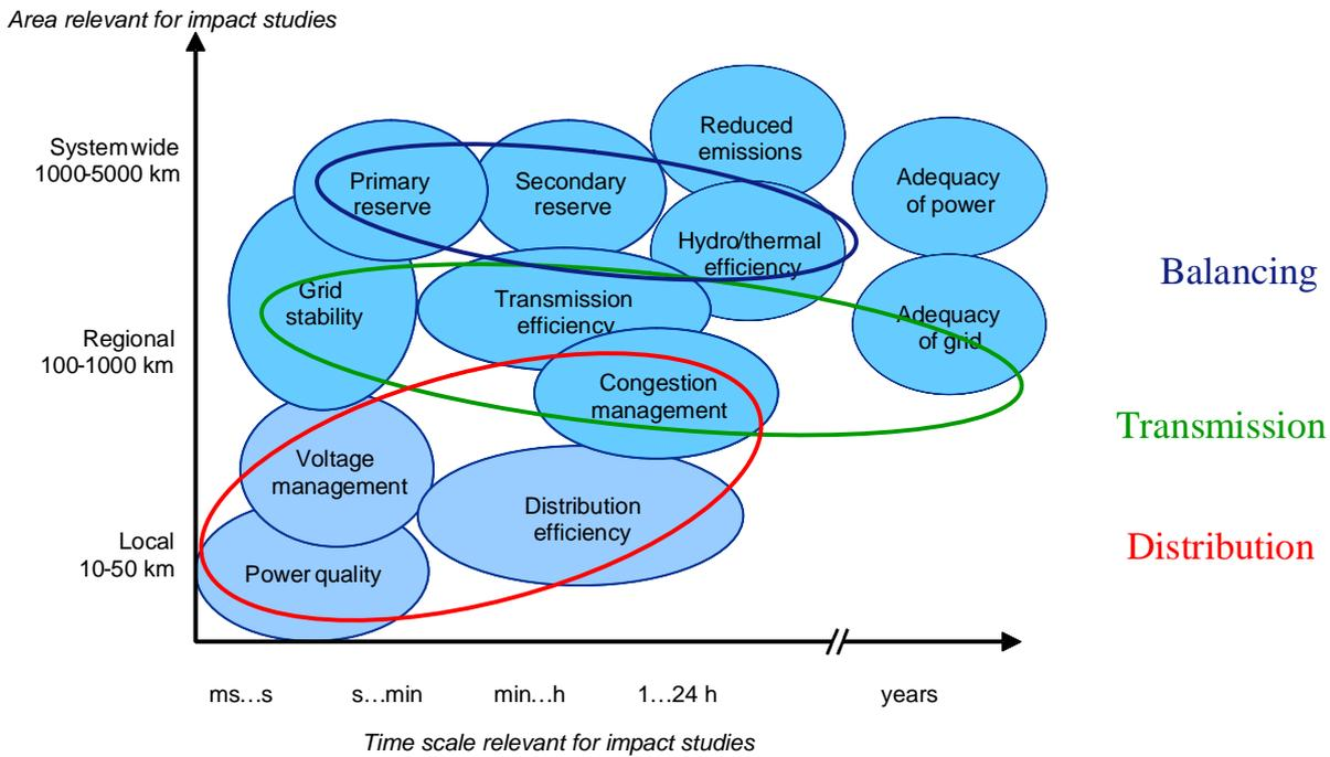
Figure 1.1. Impacts of DG on electricity system. [Hol07]
