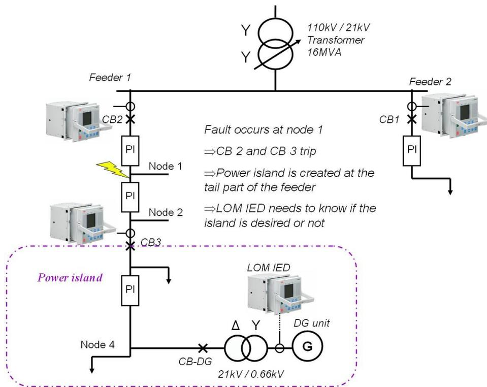
Figure 3.4. A challenge related to loss of mains protection
