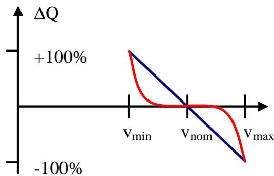
Figure 3.1. The droop characteristic (blue slope) and voltage constrained reactive power control method (red curve) of DG unit voltage controller.
