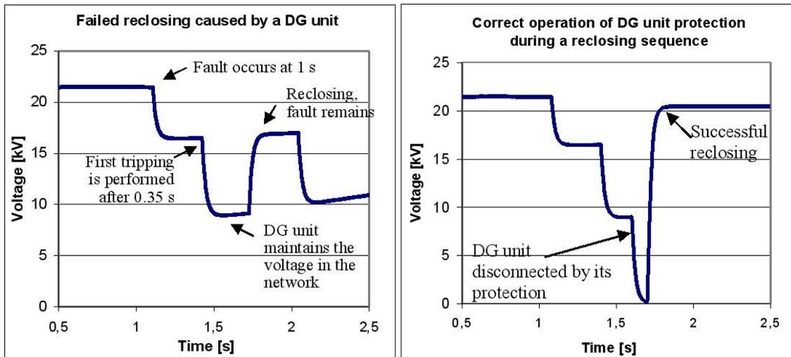
Figure 2.4. Reclosing problems caused by DG [Mäk07]
