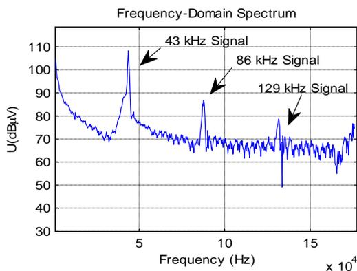
**Figure 11.** Frequency-domain spectrum computed by the IED.
