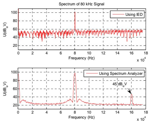
Figure 9. Spectrum analysis using IED and spectrum analyzer.
