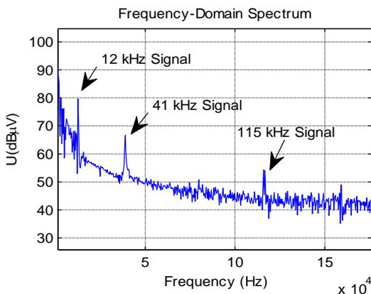
**Figure 12.** Frequency-domain spectrum computed by the IED.
