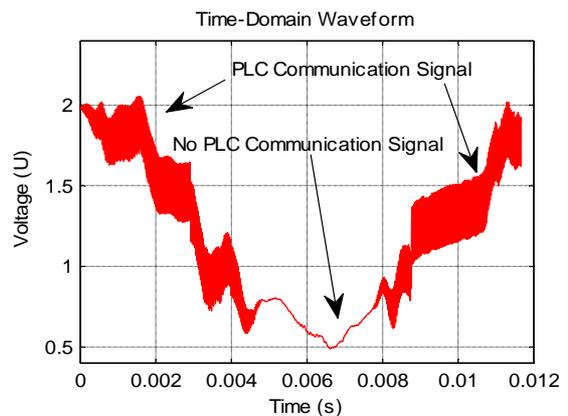
Figure 10. Time-domain waveform captured by the IED.
