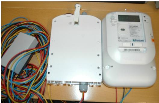
Figure 6. Smart meter and concentrator setup.
