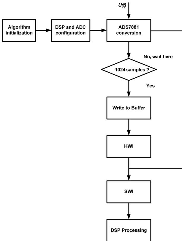
Figure 4. DSP design implementation flow of the IED.
