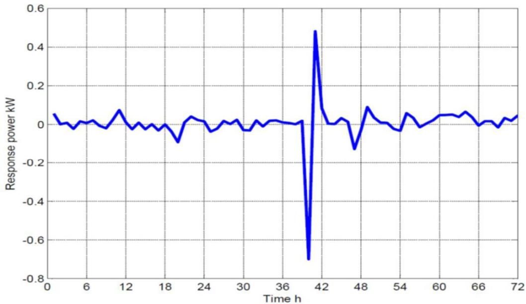
Fig.4. Daytime direct load control response identified from measured hourly powers.
