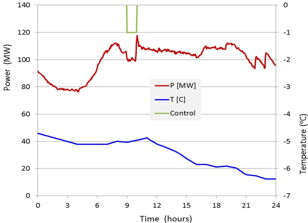
Fig. 2. Load control response in the 3 minute interval power of the distribution area in 6 Feb 2014.
