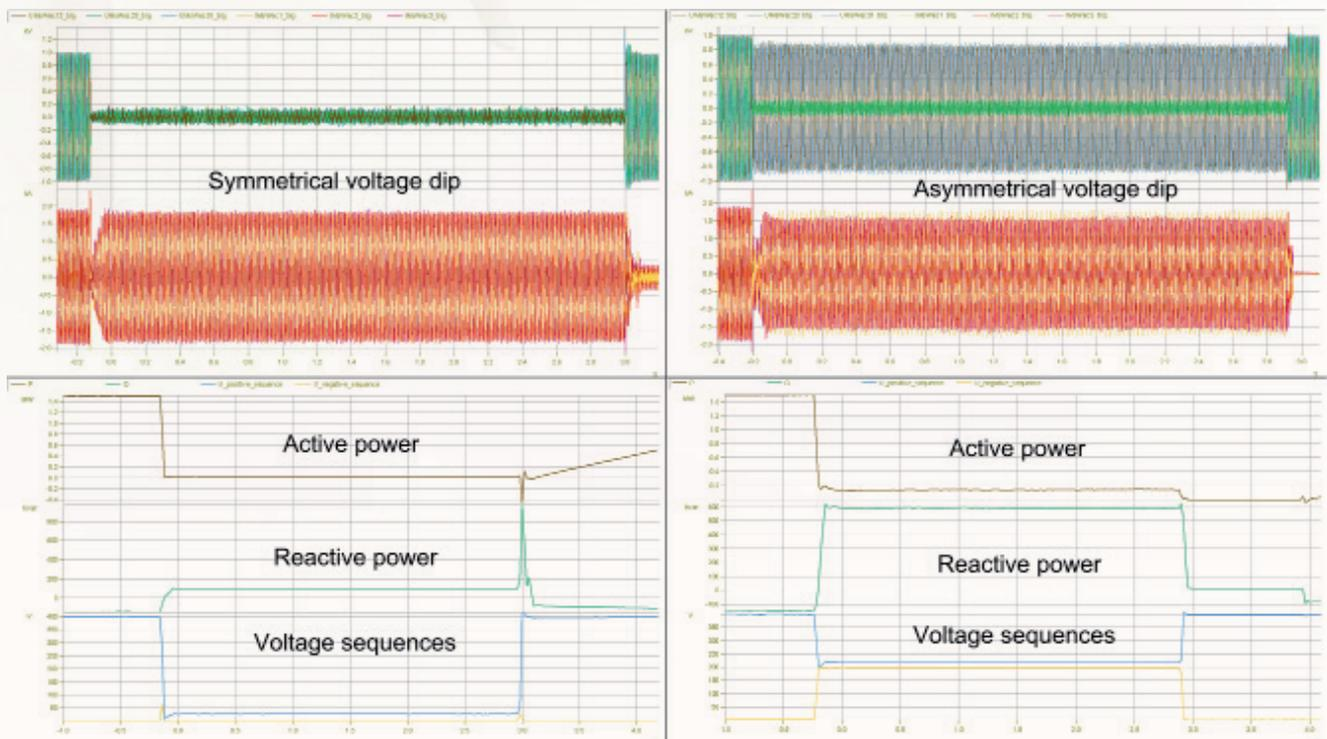
*Figure 3.* Test results show exceptional stability of the FPC. Operation here at over  $0.9 P_n$  and dip level is 0% of nominal voltage for 3 seconds
