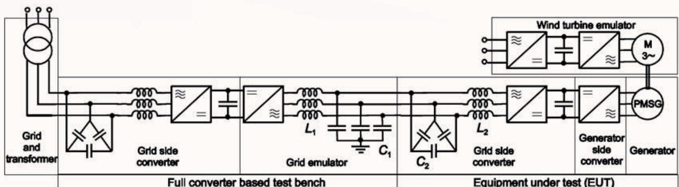
Figure 1. FRT test bench for FPCs at The Switch
