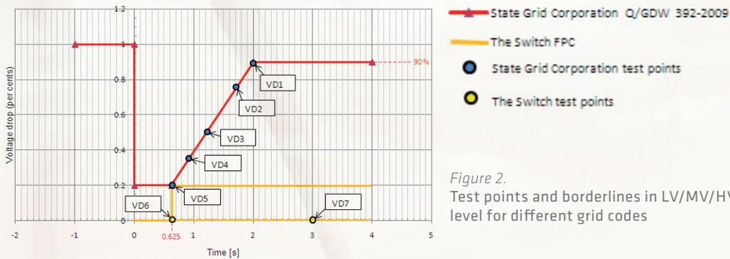
*Figure 2.* Test points and borderlines in LV/MV/HV level for different grid codes
