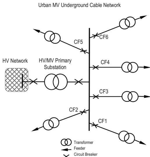
Fig. 1. The studied medium voltage cable distribution network.
