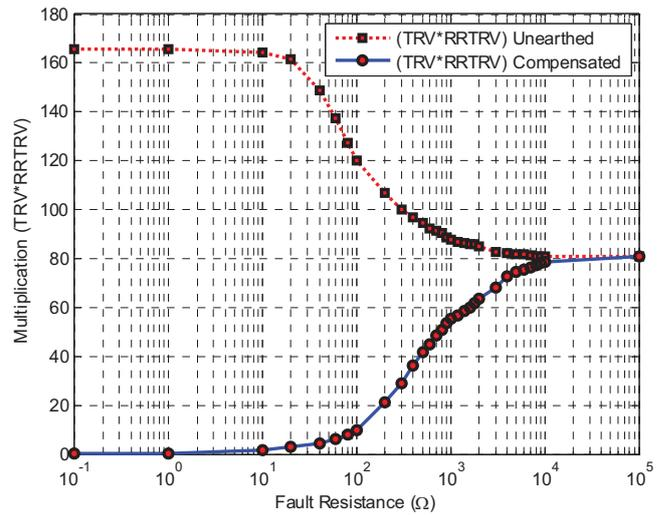
Fig. 7. The effect of the fault resistance on the multiplication (TRV\*RRTRV) in unearthed and compensated neutral networks.
