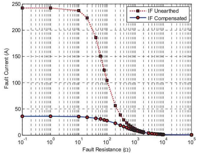
Fig. 2. The effect of the fault resistance on the fault currents in unearthed and compensated neutral networks.
