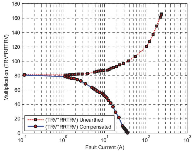
Fig. 8. The effect of the fault current on the multiplication (TRV\*RRTRV) in unearthed and compensated neutral networks, corresponding to Fig. 7.
