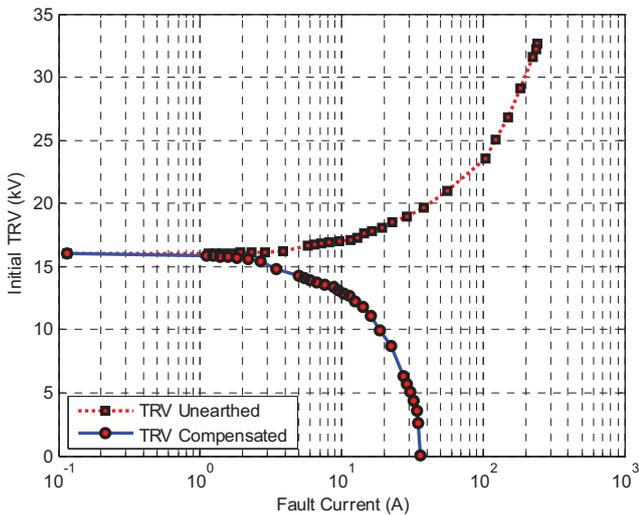
Fig. 5. The effect of the fault current on the initial TRV in unearthed and compensated neutral networks, corresponding to Fig. 3.
