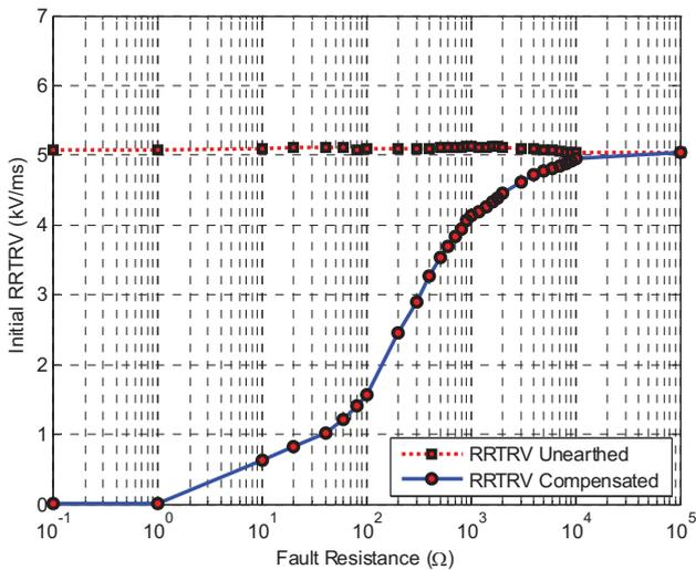
Fig. 4. The effect of the fault resistance on the initial RRTRV in unearthed and compensated neutral networks.
