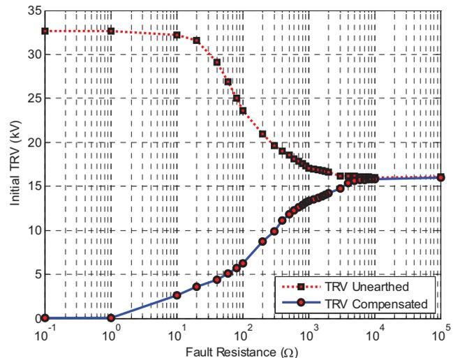
Fig. 3. The effect of the fault resistance on the initial TRV in unearthed and compensated neutral networks.
