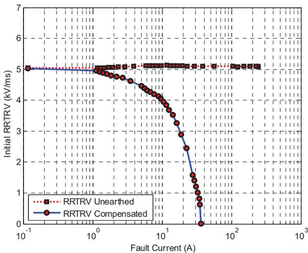
Fig. 6. The effect of the fault current on the initial RRTRV in unearthed and compensated neutral networks, corresponding to Fig. 4.
