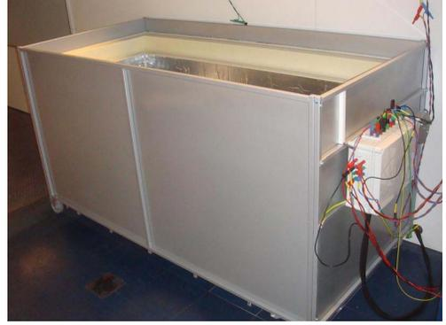
Figure 4. Balance calorimeter laboratory prototype.
