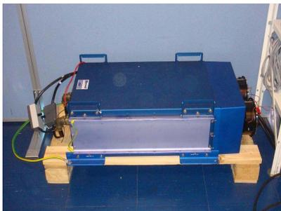
Figure 1. Maxwell BMOD0063 P125 V/63 F heavy-duty supercapacitor module.
