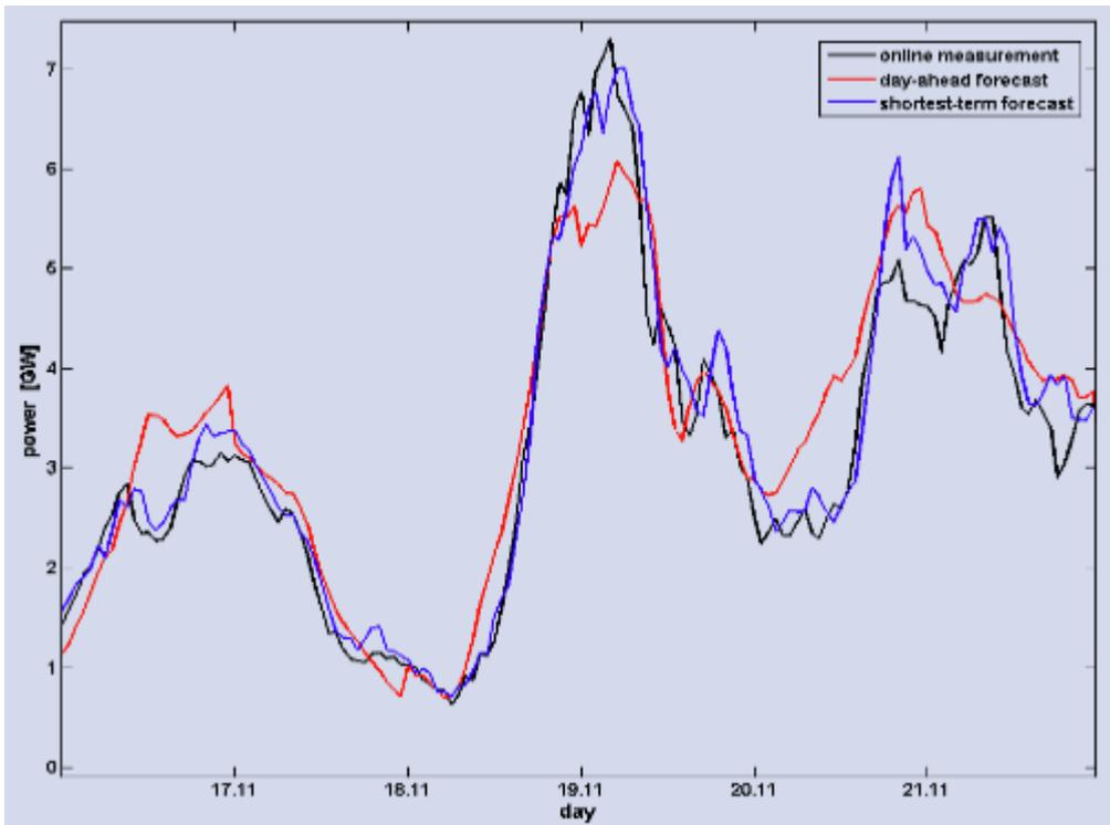
Figure 4: Feed-in of wind-generated electricity, Germany [http://windmonitor.iwes.fraunhofer.de/windwebdad/www\\_reisi\\_page\\_new.show\\_page?page\\_nr=154&lang=en](http://windmonitor.iwes.fraunhofer.de/windwebdad/www_reisi_page_new.show_page?page_nr=154&lang=en) (Data source: ISET, IWET - last update: Sep 2009)
