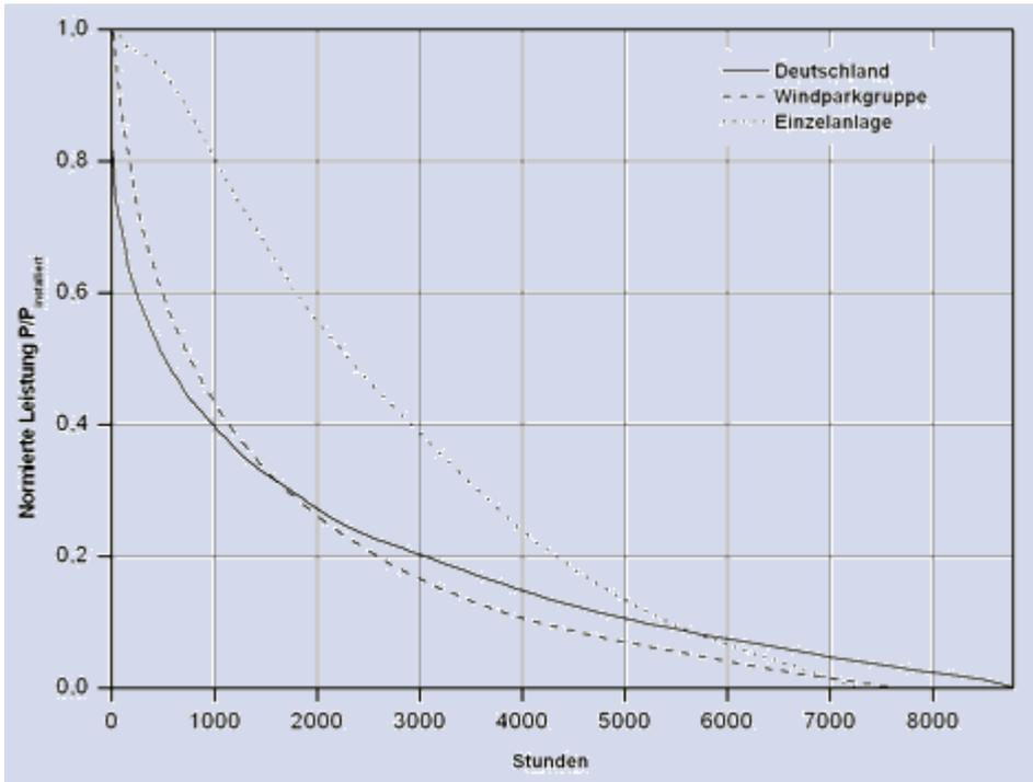
Figure 3: Wind power production versus time of utilisation in Germany. (Country – wind park – single turbine) [http://windmonitor.iwes.fraunhofer.de/windwebdad/www\\_reisi\\_page\\_new.show\\_page?page\\_nr=155&lang=en](http://windmonitor.iwes.fraunhofer.de/windwebdad/www_reisi_page_new.show_page?page_nr=155&lang=en) (Data source: ISET, IWET - last update: Feb 2006)
