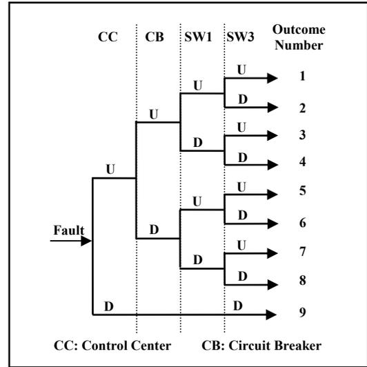
Fig. 4. An event tree that has been deduced for a typical fault shown in Fig. 2
