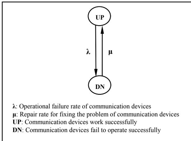
Fig. 3. A two state reliability model for representing operational failure of communication devices of the intended modules
