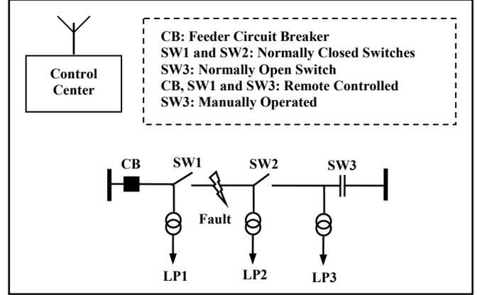
Fig. 2. An ordinary overhead line feeder equipped with an automat scheme for fault management activities.
